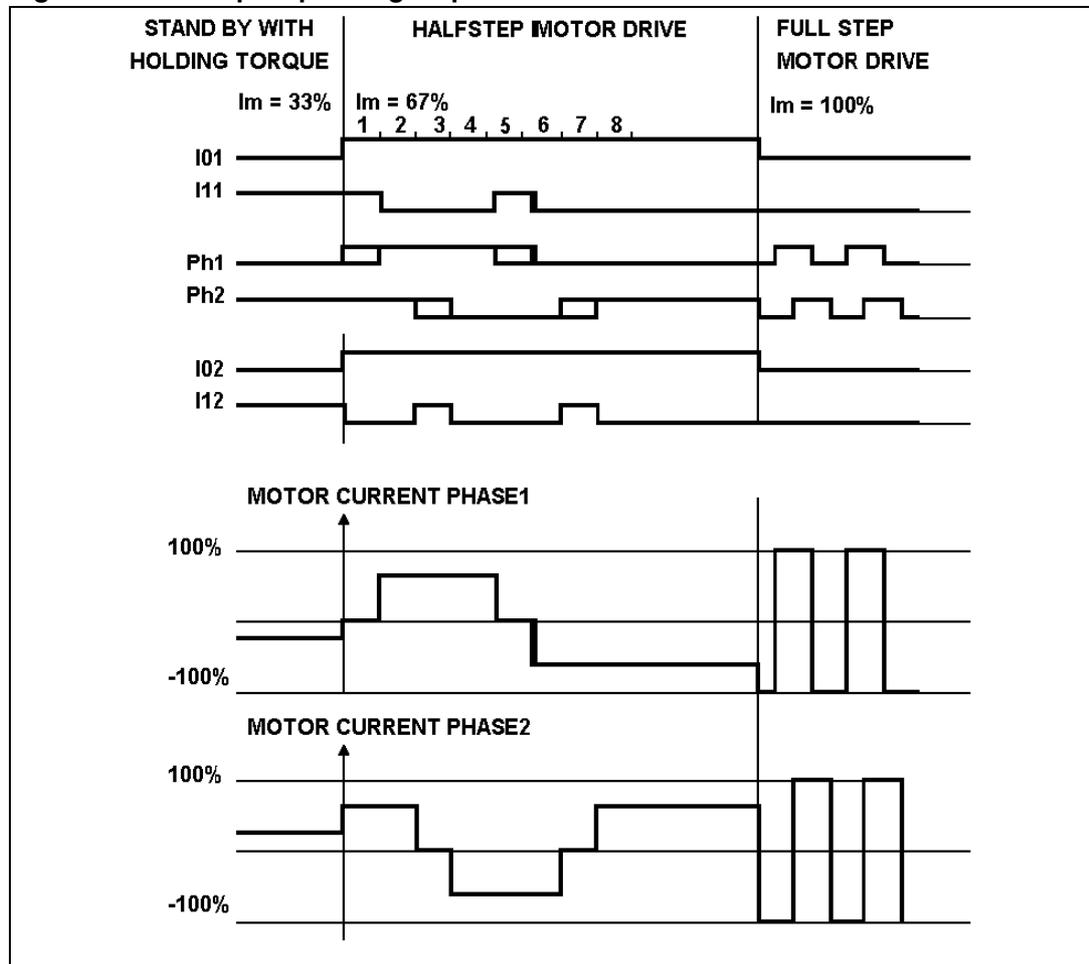
The source transistors are used to switch the power supplied to the motor winding, thus driving a constant current through the winding. It should be noted however, that is not permitted to short circuit the outputs.
