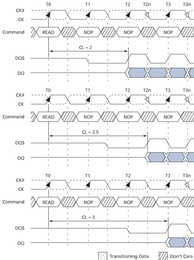
Note: BL = 4 in the cases shown; shown with nominal  $t_{AC}$ ,  $t_{DQCK}$ , and  $t_{DQSQ}$ .
