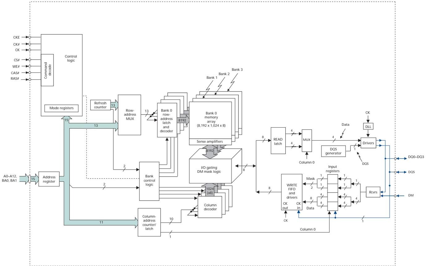
Figure 4: 32 Meg x 8 Functional Block Diagram
