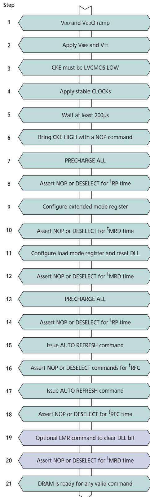
Figure 22: INITIALIZATION Timing Diagram
