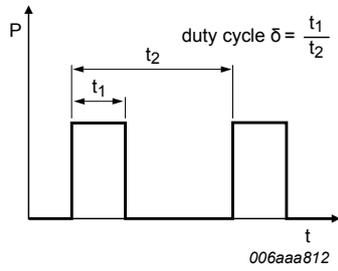
Fig. 17. Duty cycle definition
