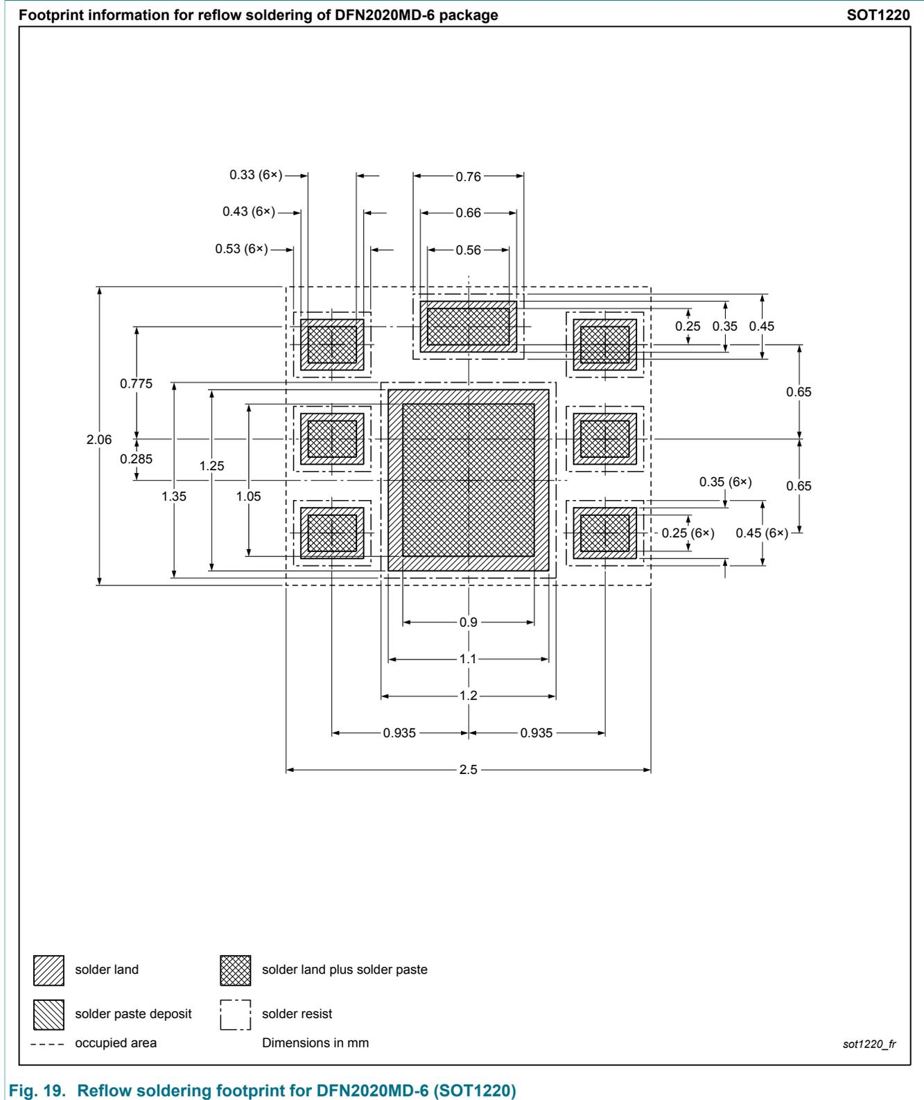
Fig. 19. Reflow soldering footprint for DFN2020MD-6 (SOT1220)
