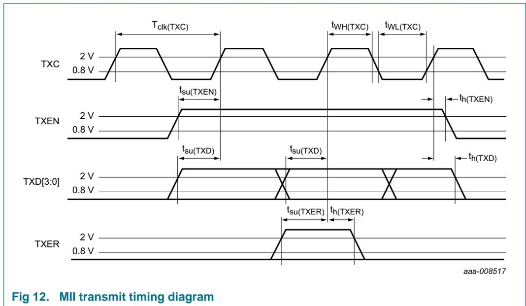
**Fig 12. MII transmit timing diagram**
