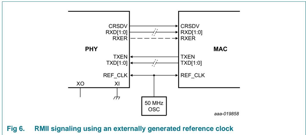
Fig 6. RMII signaling using an externally generated reference clock
