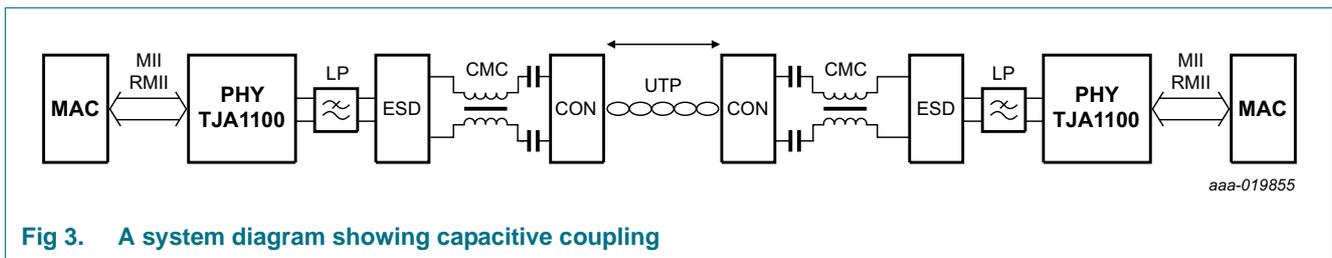
Fig 3. A system diagram showing capacitive coupling
