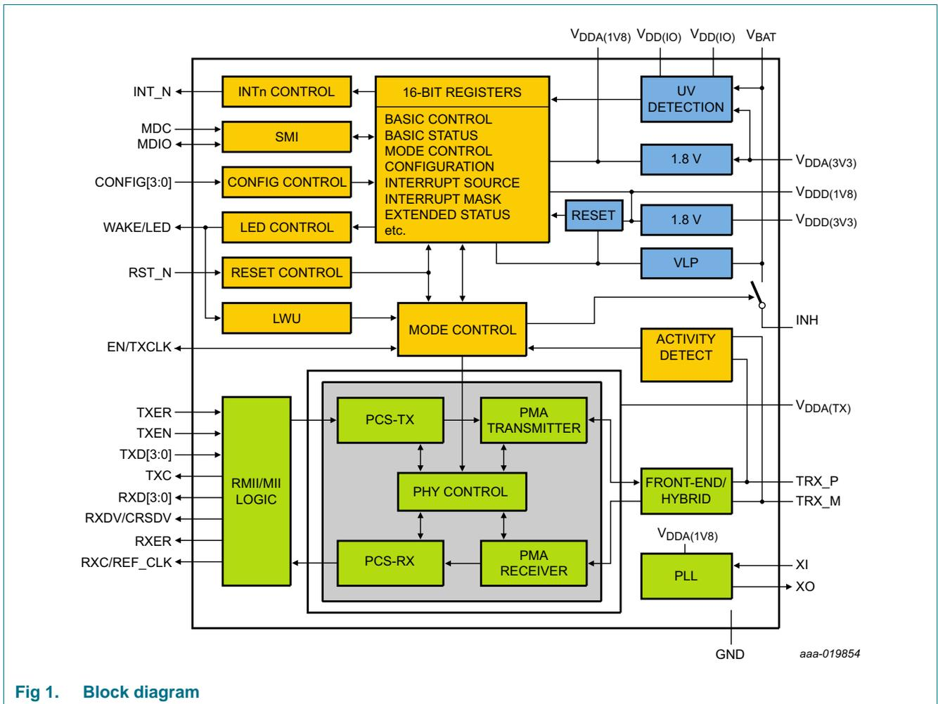
Fig 1. Block diagram
