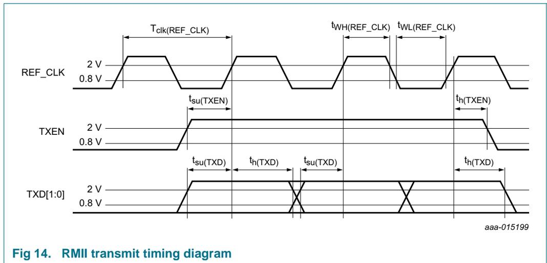
Fig 14. RMII transmit timing diagram
