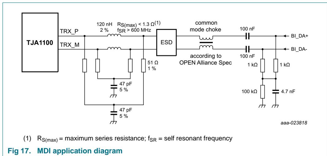
It is advised to use a PESD2ETH diode to protect against shorts to bus lines greater than 5 V. The supply terminal of the diode should be connected to a 3.3 V domain that is available when the TJA1100 is active. The diode layout should be symmetrical, as shown in the routing scheme example in [Figure 18](#).
