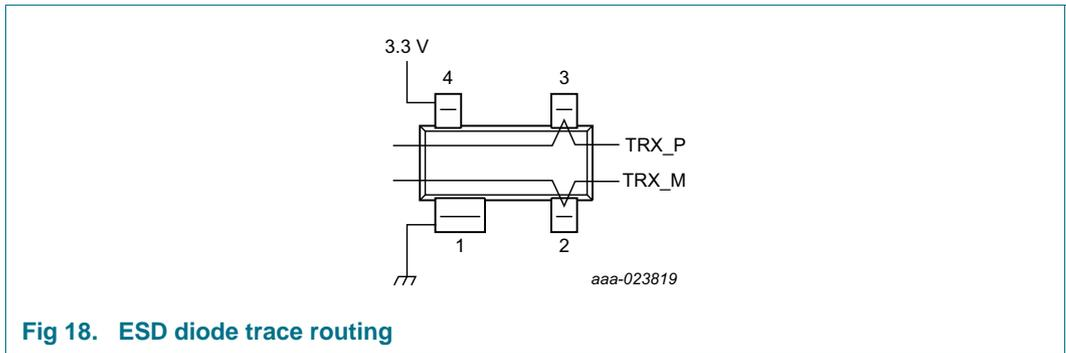
Fig 18. ESD diode trace routing
