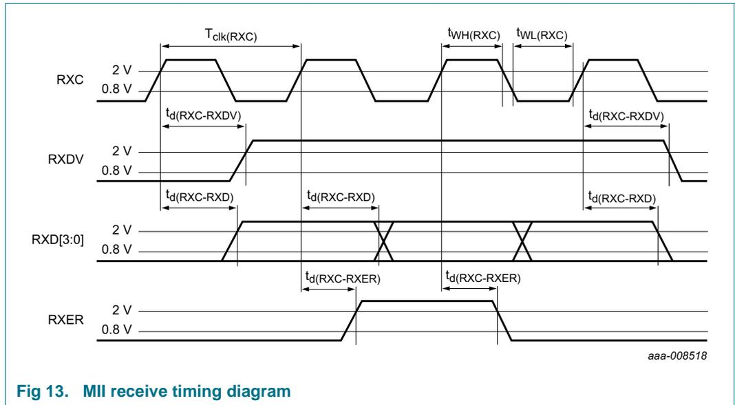
Fig 13. MII receive timing diagram
