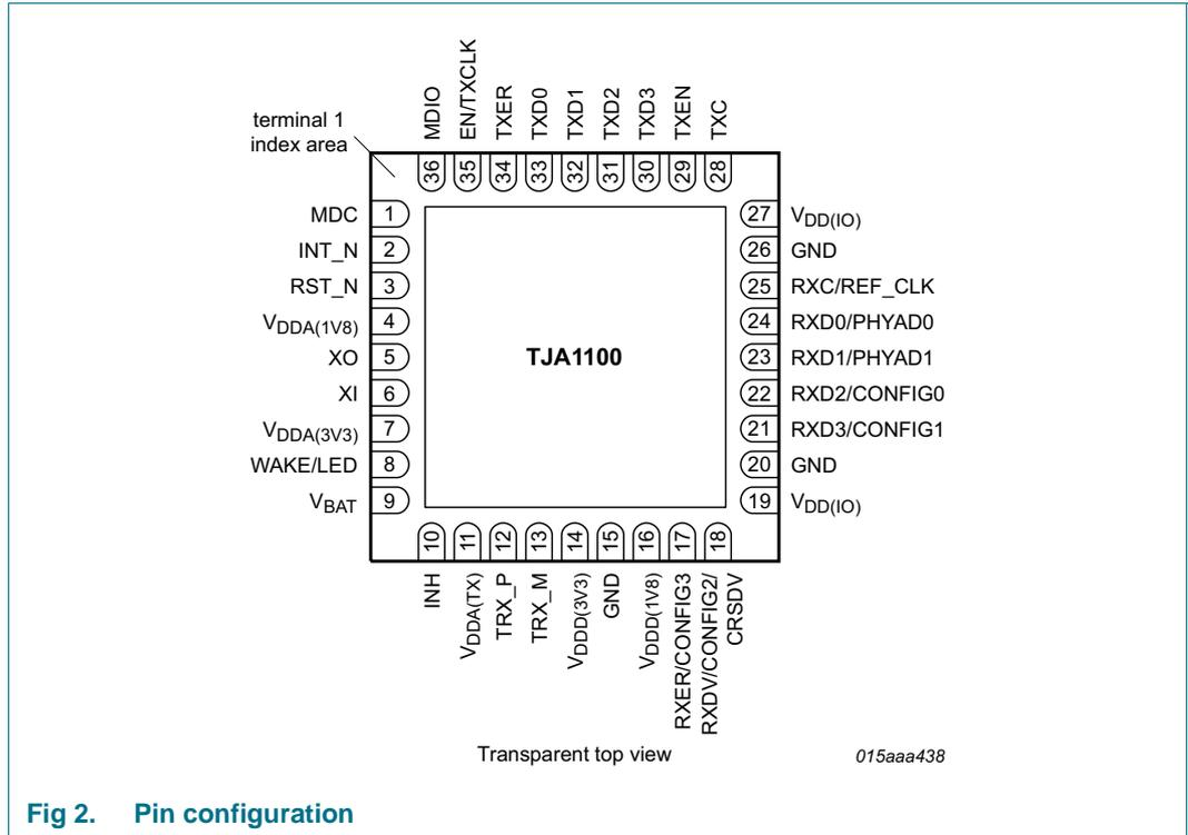
Fig 2. Pin configuration
