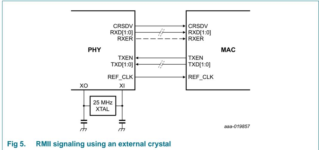
Fig 5. RMII signaling using an external crystal
