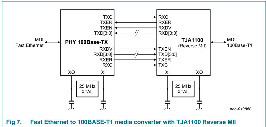
Fig 7. Fast Ethernet to 100BASE-T1 media converter with TJA1100 Reverse MII
