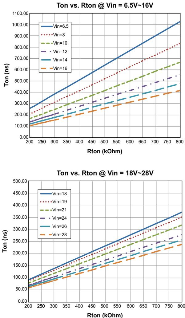
Figure 3. Ton vs. Rton Curves for AOZ2255EQI-30
