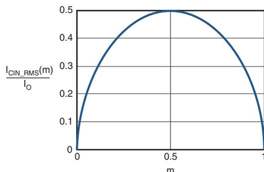
Figure 4. I<sub>CIN</sub> vs. Voltage Conversion Ratio
