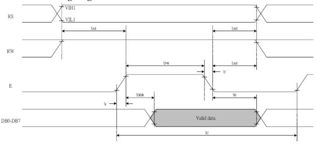
Write cycle (Ta=25°C, VDD=5.0V)
