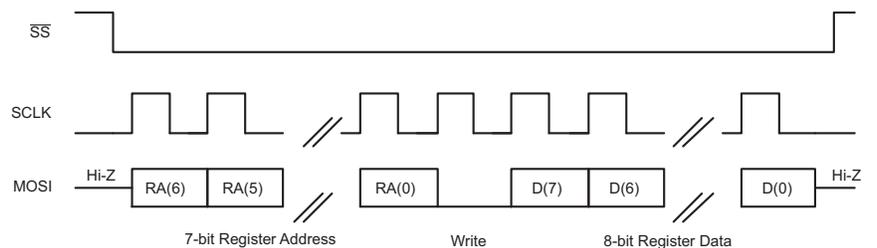
Figure 84. SPI Single-Byte Write Transfer
