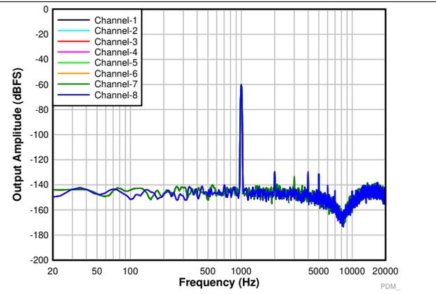
Fourth order PDM modulator with  $PDMCLKx = 3.072\text{ MHz}$
