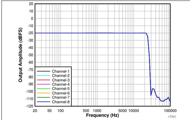
Fourth order PDM modulator with  $PDMCLKx = 3.072\text{ MHz}$
