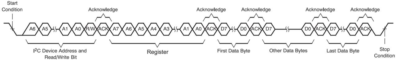
**Figure 81. I<sup>2</sup>C Multiple-Byte Write Transfer**
