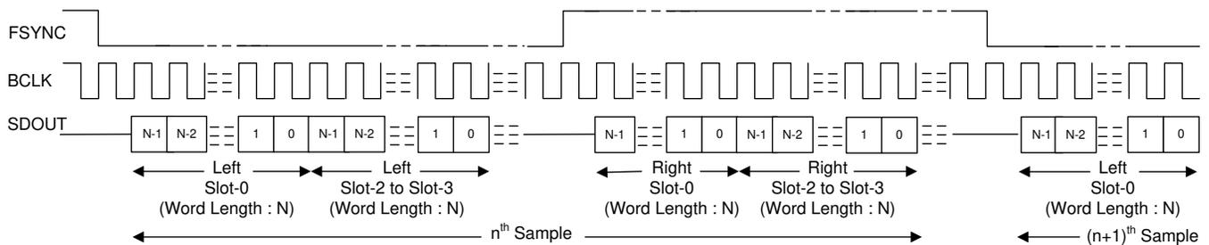
Figure 24. I²S Protocol Timing (TX\_OFFSET = 0 and BCLK\_POL = 1)
