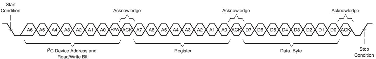
Figure 80. I<sup>2</sup>C Single-Byte Write Transfer
