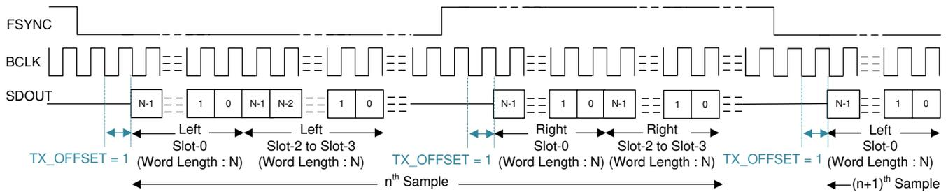
Figure 22. I²S Protocol Timing (TX\_OFFSET = 1)
