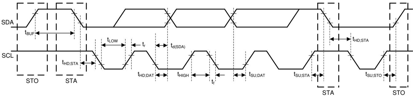
Figure 1. I<sup>2</sup>C Interface Timing Diagram
