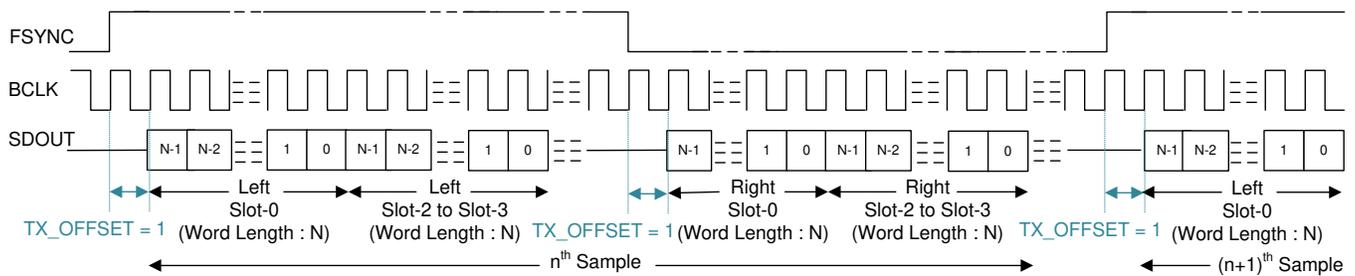
Figure 28. LJ Protocol Timing ( $TX\_OFFSET = 1$  and  $BCLK\_POL = 1$ )
