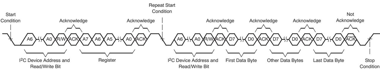
**Figure 83. I<sup>2</sup>C Multiple-Byte Read Transfer**
