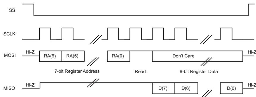
Figure 85. SPI Single-Byte Read Transfer
