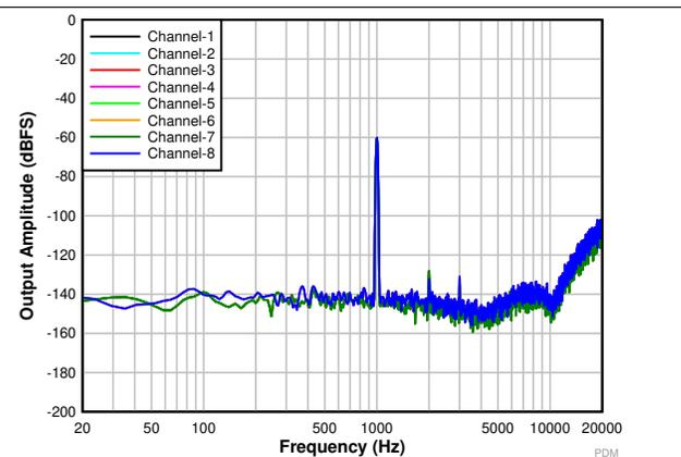
Fourth order PDM modulator with  $PDMCLKx = 1.536\text{ MHz}$
