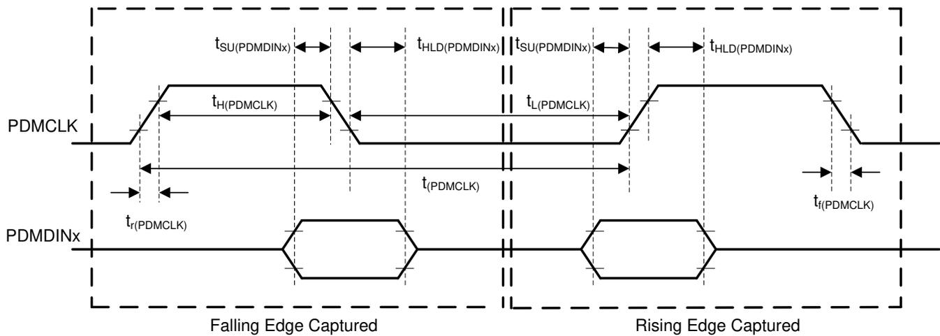
**Figure 4. PDM Digital Microphone Interface Timing Diagram**
