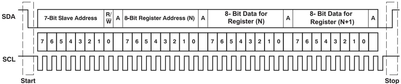
Figure 79. Typical I<sup>2</sup>C Sequence
