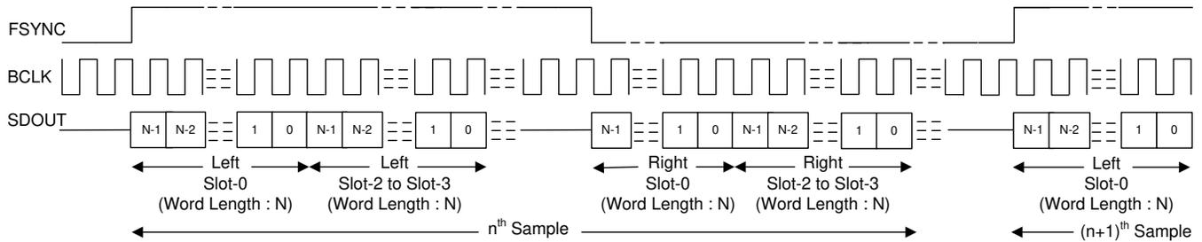
Figure 25. LJ Mode Standard Protocol Timing ( $TX\_OFFSET = 0$ )
