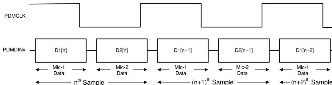
Figure 31. Digital PDM Microphone Protocol Timing Diagram
