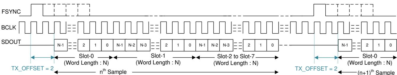
**Figure 18. TDM Mode Protocol Timing (TX\_OFFSET = 2)**
