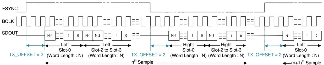
Figure 26. LJ Protocol Timing ( $TX\_OFFSET = 2$ )
