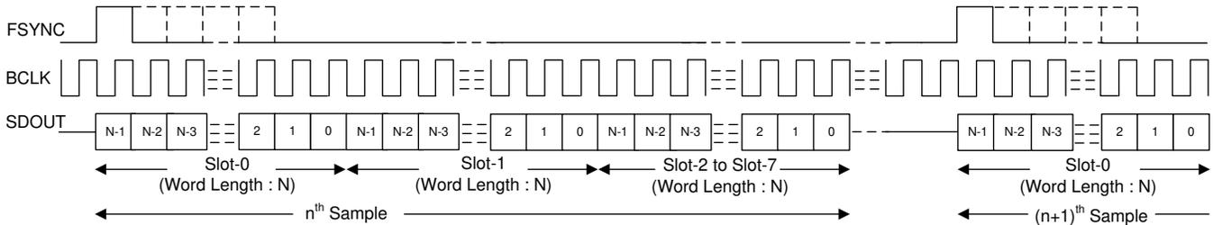
Figure 20. TDM Mode Protocol Timing (TX\_OFFSET = 0 and BCLK\_POL = 1)
