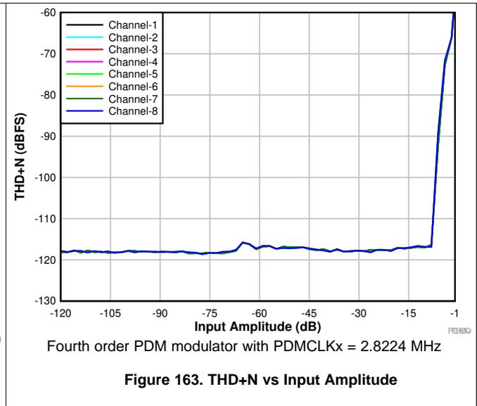
Figure 163. THD+N vs Input Amplitude
