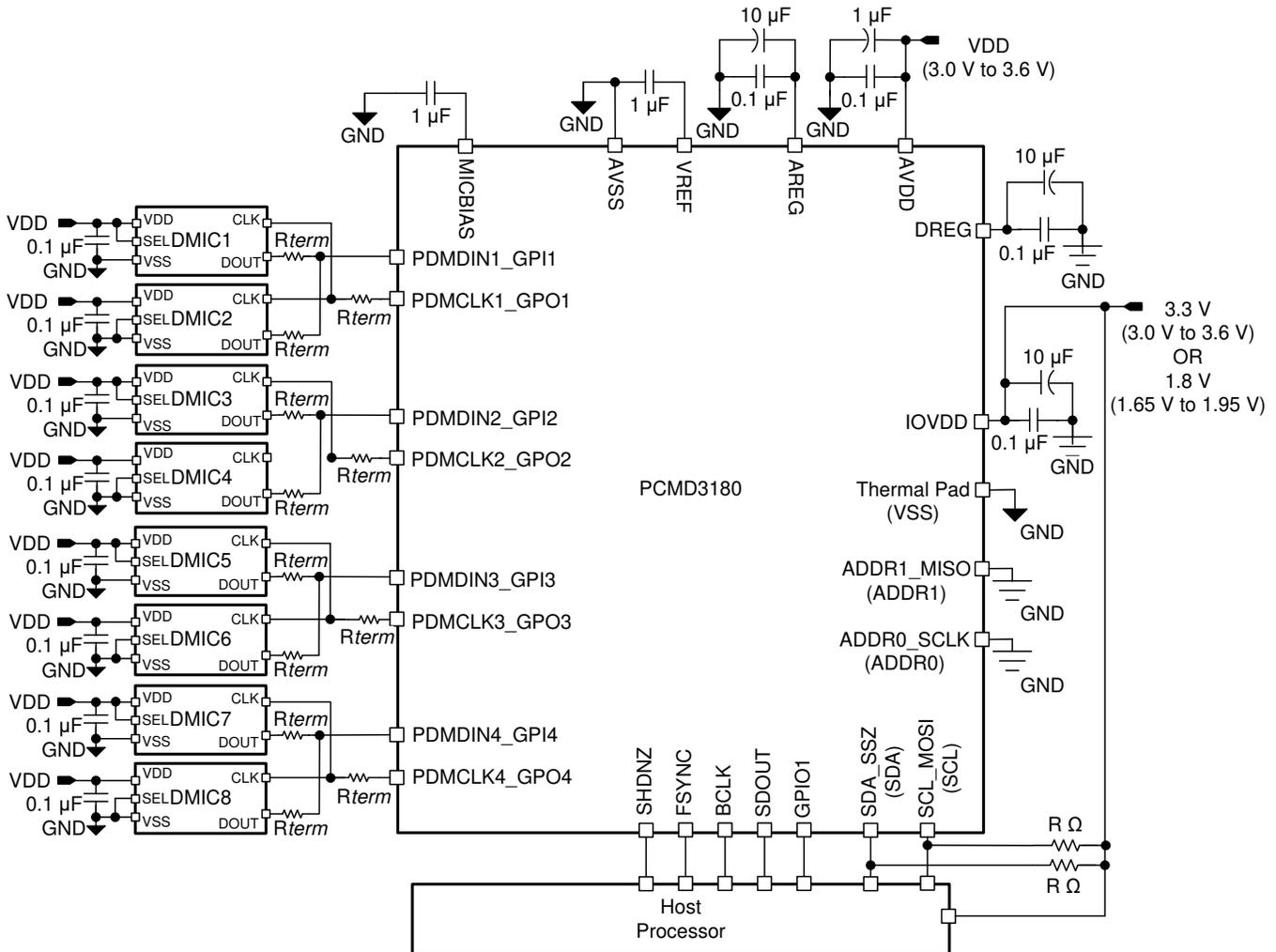
Figure 161. Eight-Channel Digital PDM Microphone Recording Diagram
