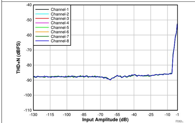
Fourth order PDM modulator with  $PDMCLKx = 1.536\text{ MHz}$
