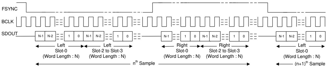
Figure 21. I<sup>2</sup>S Mode Standard Protocol Timing (TX\_OFFSET = 0)
