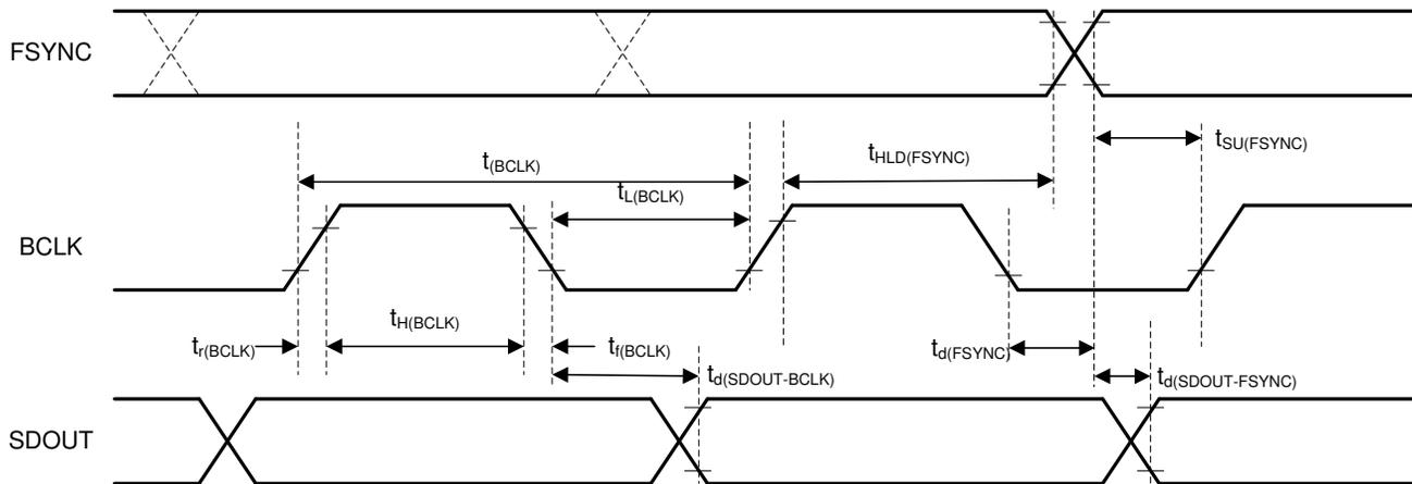
**Figure 3. TDM (With BCLK\_POL = 1), I<sup>2</sup>S, and LJ Interface Timing Diagram**
