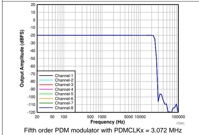
Figure 7. Frequency Response With a -20-dBr Input
