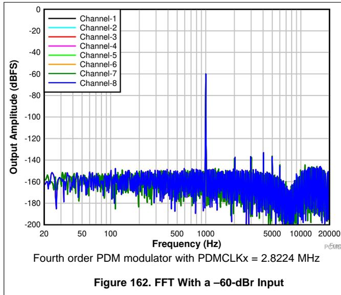
Figure 162. FFT With a -60-dBr Input
