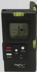
DWL 1000XY is a 2-Axis digital post level, having a resolution of 0.05°, designed for professional & tradesmen to achieve speedy and accurate means of putting up post, fences/guttering, pipe, window, and door frames.
