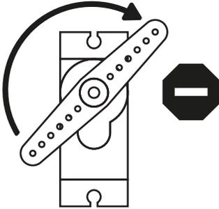
Connect a horn to the servo axle and gently rotate clockwise until it stops. Then rotate back an 1/8 turn.
