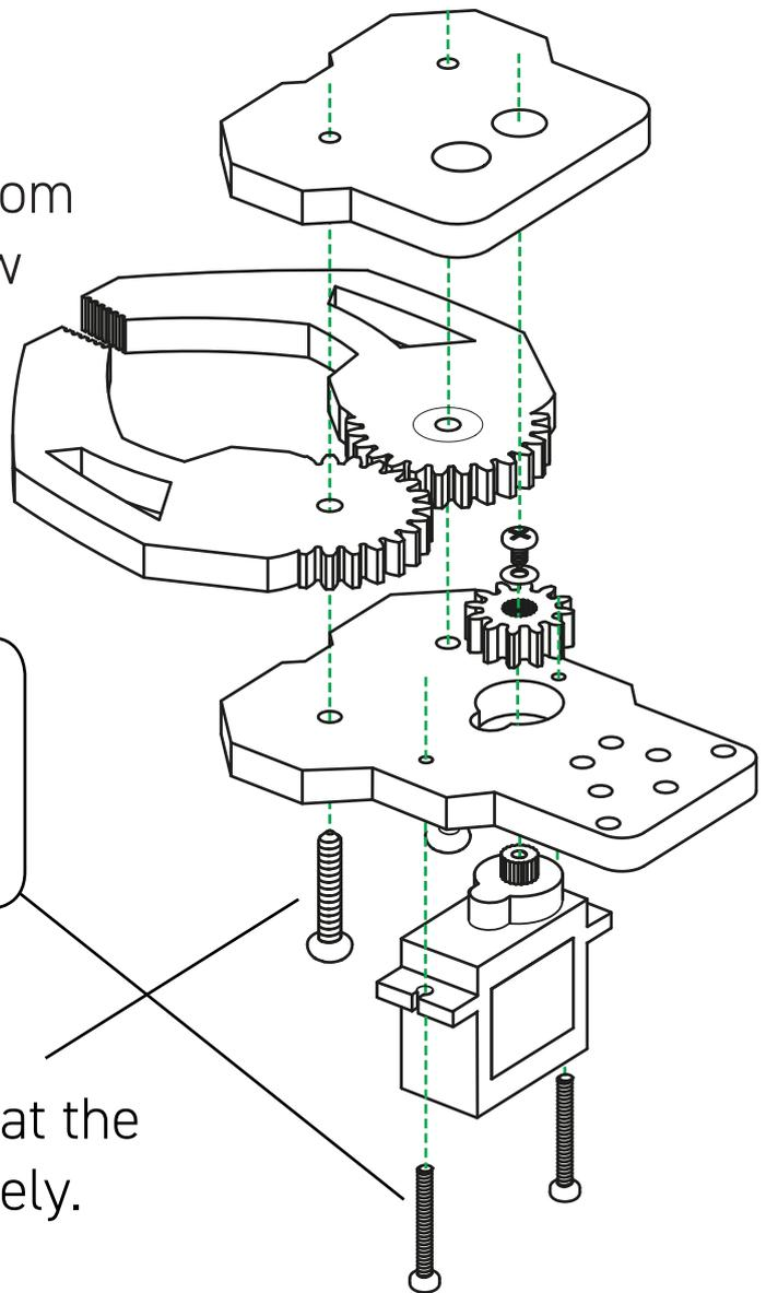
Take care not to damage the servos wires when tightening these screws!
