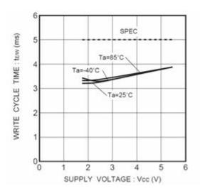
Figure 31. Write cycle time tE/W
