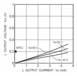
Figure 5. L output voltage VOL-IOL (Vcc=2.5V)
