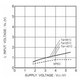
Figure 3. L input voltage VIL (CS,SK,DI)
