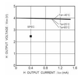
Figure 9. H output voltage VOH-IOH (Vcc=4.0V)
