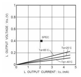
Figure 6. L output voltage VOL-IOL (Vcc=4.0V)
