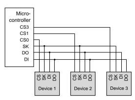
Figure 32-(a) Connection by 4 lines
