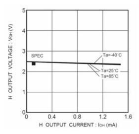
Figure 8. H output voltage VOH-IOH (Vcc=2.5V)
