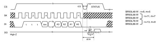
Figure 37. Erase cycle timing
