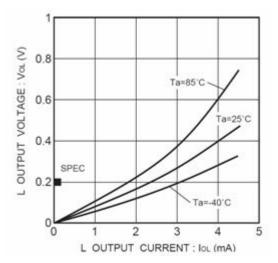
Figure 4. L output voltage VOL-IOL (Vcc=1.8V)
