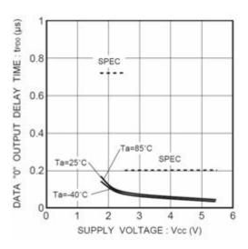
Figure 27. Data "0" output delay time tPD0
