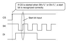
Figure 43. Normal action timing
