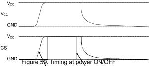
(Bad example) CS pin is pulled up to Vcc.
