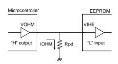
Figure 48. CS pull down resistance
