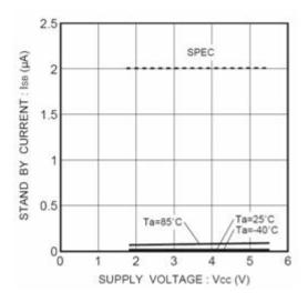
Figure 18. Consumption current at standby action ISB
