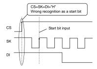
Figure 42. Wrong action timing
