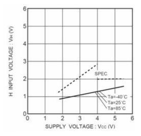
Figure 2. H input voltage VIH (CS,SK,DI)
