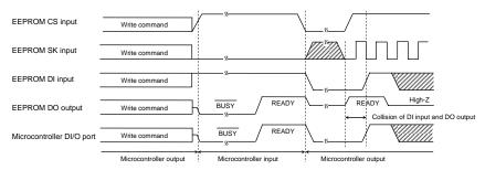
Figure 55. Collision timing at DI, DO direct connection
