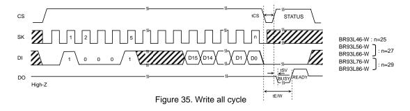
OIn this command, input 16bit data is written simultaneously to all adresses. Data is not written continuously per one word but is written in bulk, the write time is only Max. 5ms in conformity with tE/W.
