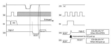
Figure 49. READY output timing at DO=OPEN
