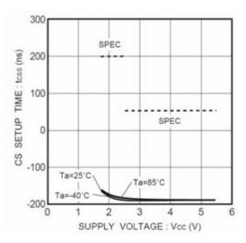
Figure 24. CS setup time tCSS
