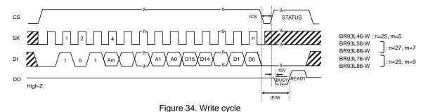
OIn this command, input 16bit data (D15 to D0) are written to designated addresses (Am to A0). The actual write starts by the fall of CS of D0 taken SK clock.
