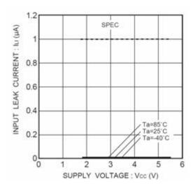
Figure 10. Input leak current ILI (CS,SK,DI)
