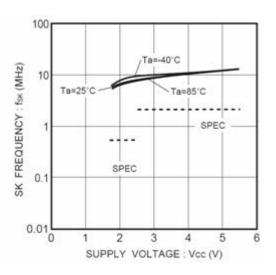
Figure 19. SK frequency fSK
