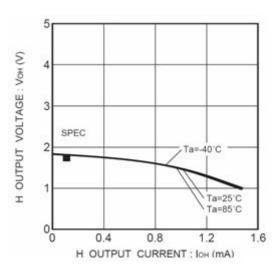
Figure 7. H output voltage VOH-IOH (Vcc=1.8V)
