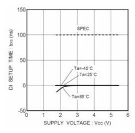
Figure 26. DI setup time tDIS
