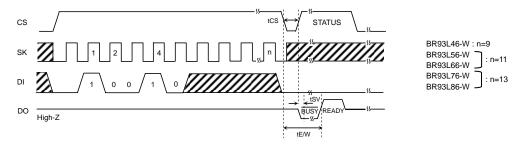
Figure 38. Chip erase cycle timing
