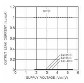
Figure 11. Output leak current ILO (DO)
