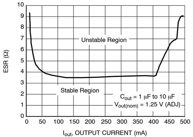
Figure 20. Output Capacitor ESR Stability vs. Output Current
