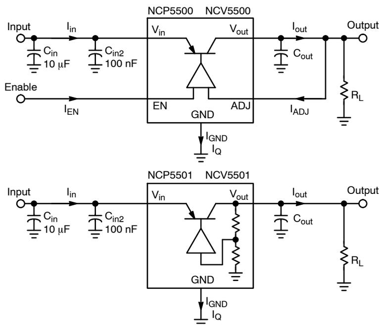
Figure 21. Measuring Circuits
