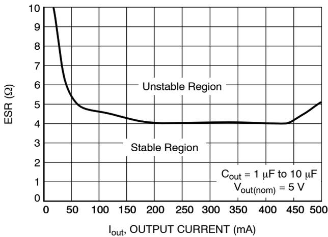
Figure 17. Output Capacitor ESR Stability vs. Output Current
