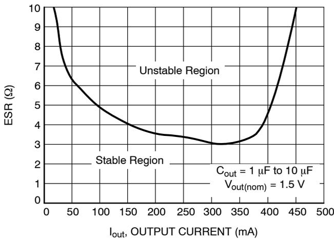
Figure 19. Output Capacitor ESR Stability vs. Output Current
