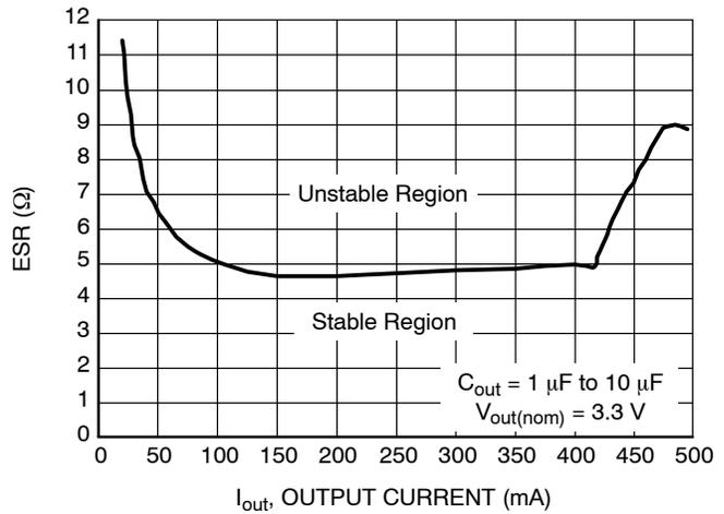
Figure 18. Output Capacitor ESR Stability vs. Output Current
