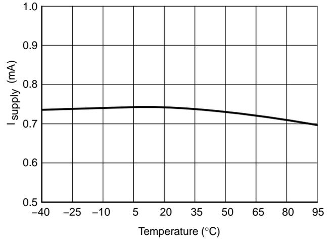
Figure 3. Typical Supply Current vs. Temperature
