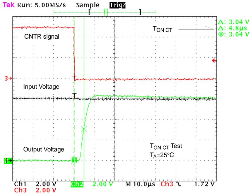
Figure 16. T<sub>ON CT</sub> Waveforms
