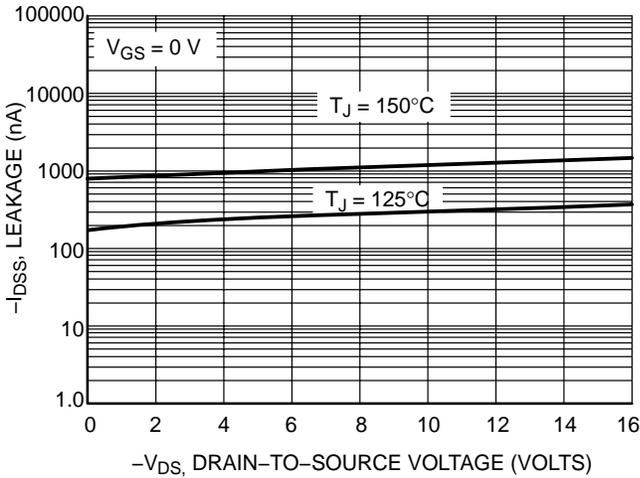
Figure 10. Drain-to-Source Leakage Current vs. Voltage
