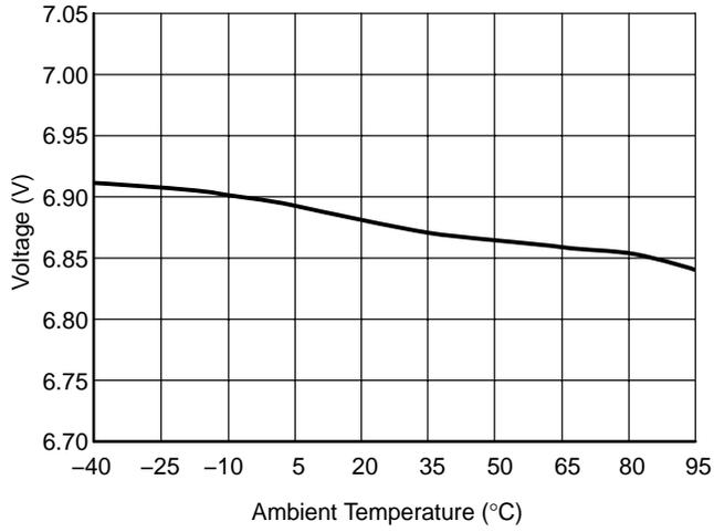
Figure 2. Typical  $V_{th}$  Threshold Variation vs. Temperature
