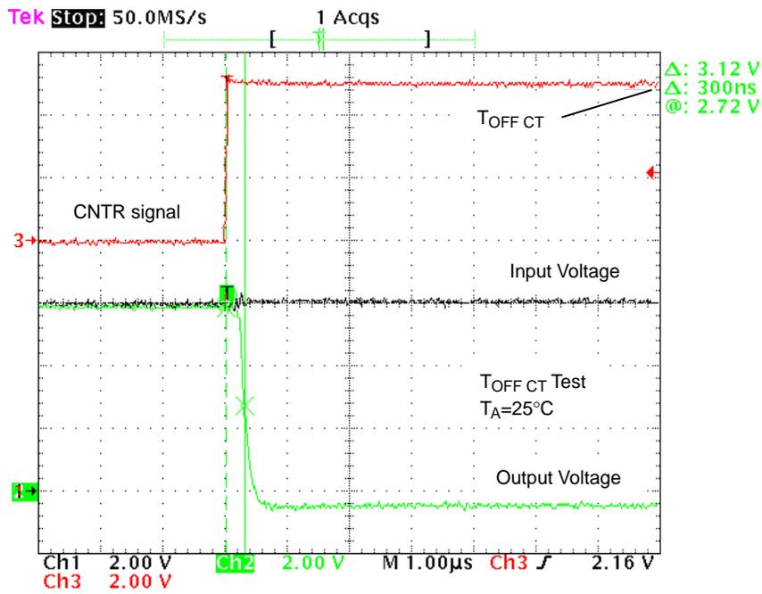
Figure 17. T<sub>OFF CT</sub> Waveforms
