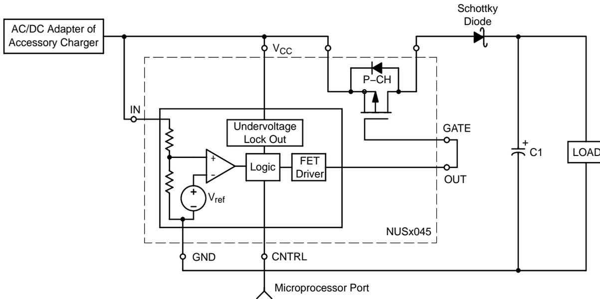
Figure 1. Simplified Schematic
