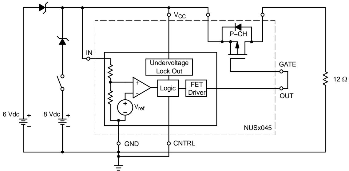
Figure 12. Test Circuit for  $T_{ON IN}$  and  $T_{OFF IN}$
