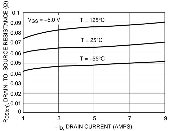
Figure 9. On-Resistance vs. Drain Current and Temperature
