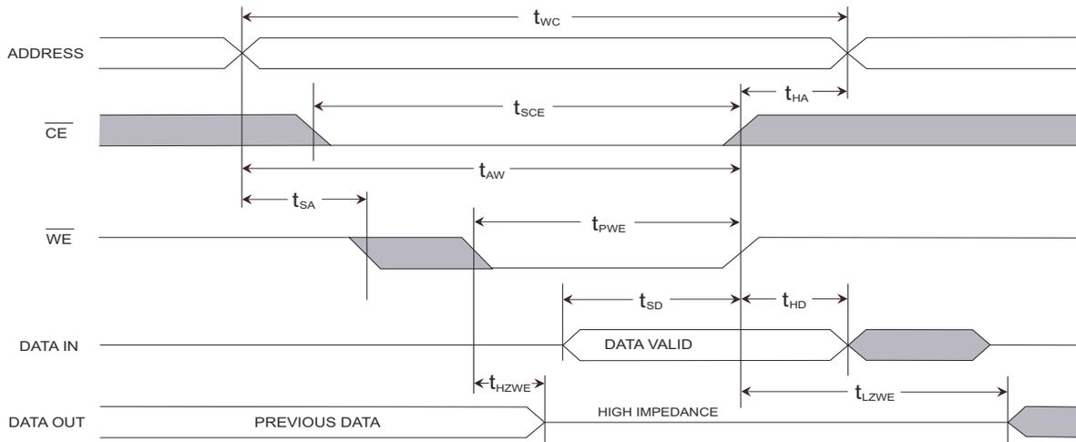
Figure 8. SRAM Write Cycle 2:  $\overline{CE}$  Controlled <sup>[9]</sup>
