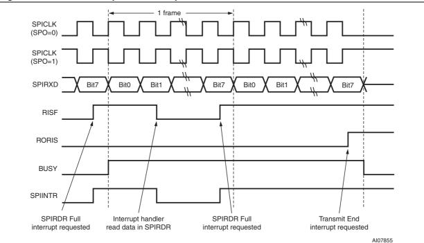
Figure 42. SPI Receive operation example
