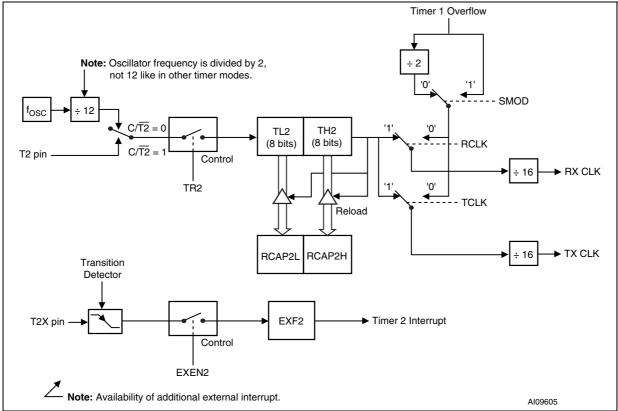
Figure 26. Timer 2 in baud rate generator mode
