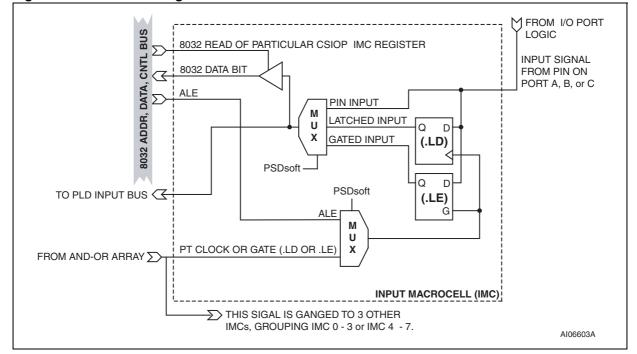
Figure 67. Detail of a single IMC
