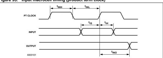
Figure 93. Input macrocell timing (product term clock)
