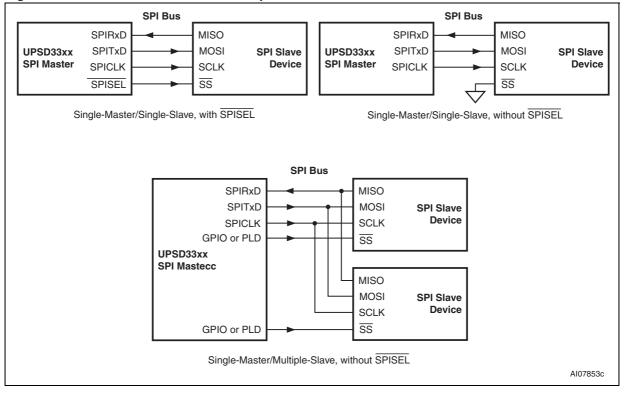
Figure 40. SPI device connection examples
