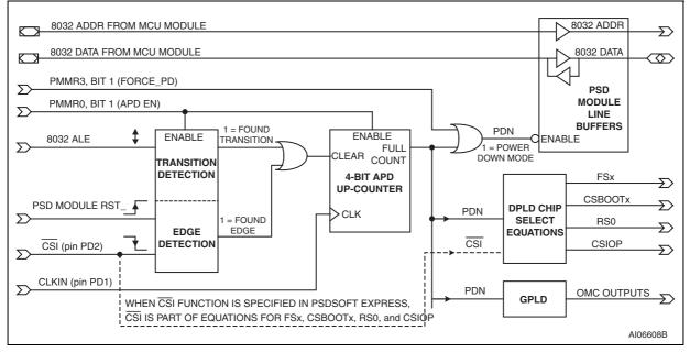
Figure 78. Power-down mode flowchart
