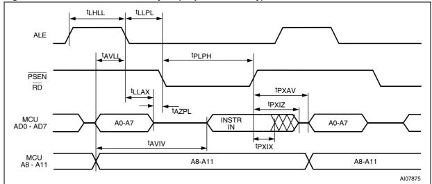
Figure 87. External **PSEN**/READ cycle (80-pin device only)
