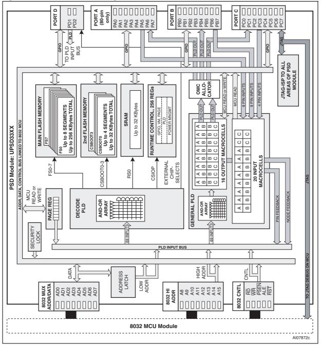
Figure 50. PSD module block diagram
