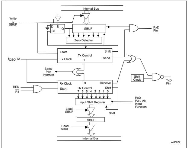
Figure 27. UART mode 0, block diagram
