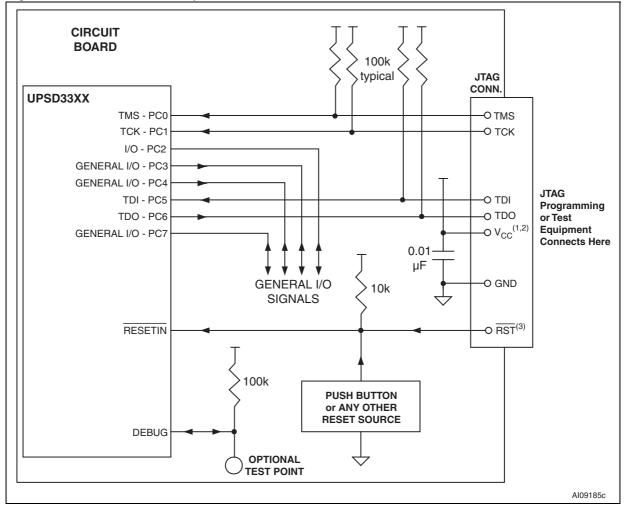
Figure 80. Recommended 4-pin JTAG connections
