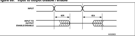
Figure 89. Input to output disable / enable
