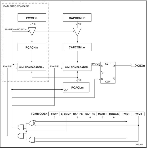
Figure 49. PWM mode - (x8) programmable frequency
