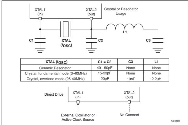
Figure 14. Oscillator and clock connections
