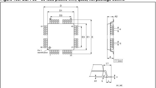
Figure 103. LQFP80 – 80-lead plastic thin, quad, flat package outline
