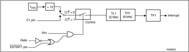
Figure 22. Timer/Counter Mode 2: 8-bit Auto-reload
