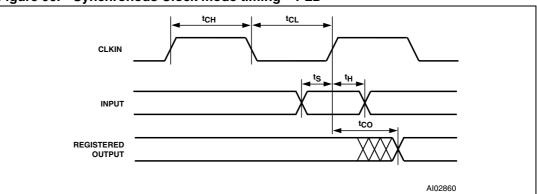
Figure 90. Synchronous Clock mode timing – PLD
