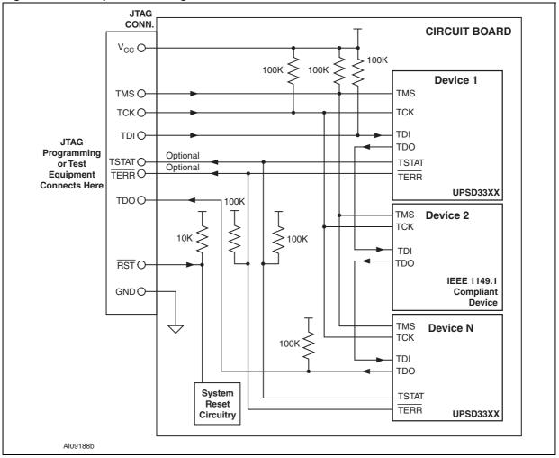
Figure 83. Example of chaining UPSD33xx devices
