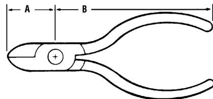
Leverage ratio is obtained by dividing dimension A into dimension B.
