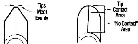
A precision tip interface assures clean cutting of fine wires, while the "no contact" area behind the tips extends cutter life by allowing the tips to continue to meet as they wear.
