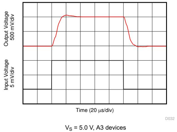
Figure 6-22. Step Response (10-mV<sub>PP</sub> Input Step)
