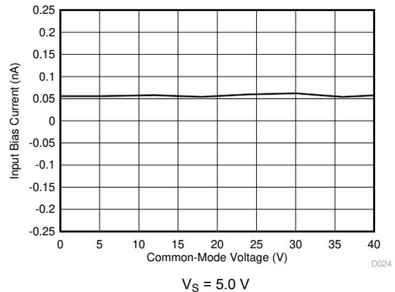
**Figure 6-14. Input Bias Current vs. Common-Mode Voltage**
