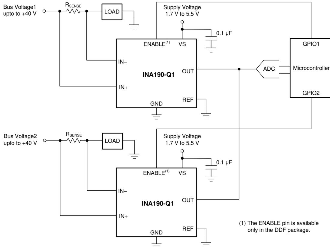
**Figure 7-5. Multiplexing Multiple Devices With the ENABLE Pin**
