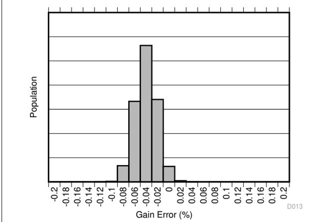
**Figure 6-5. Gain Error Production Distribution**
