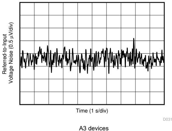
Figure 6-21. 0.1-Hz to 10-Hz Voltage Noise (Referred-To-Input)
