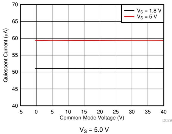
Figure 6-19. Quiescent Current vs. Common Mode Voltage
