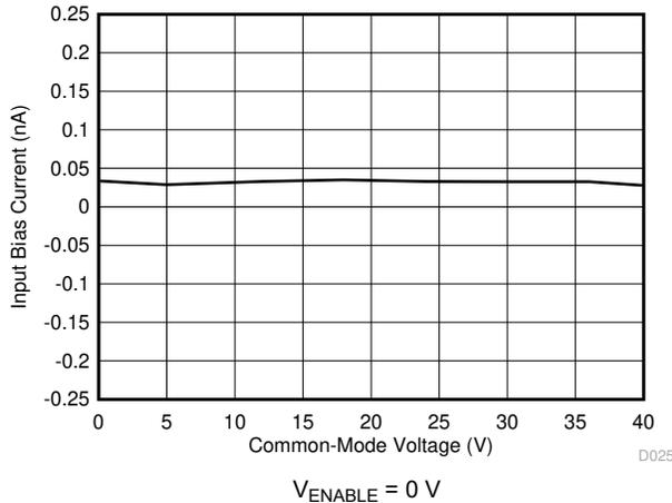
**Figure 6-15. Input Bias Current vs. Common-Mode Voltage (Shutdown)**
