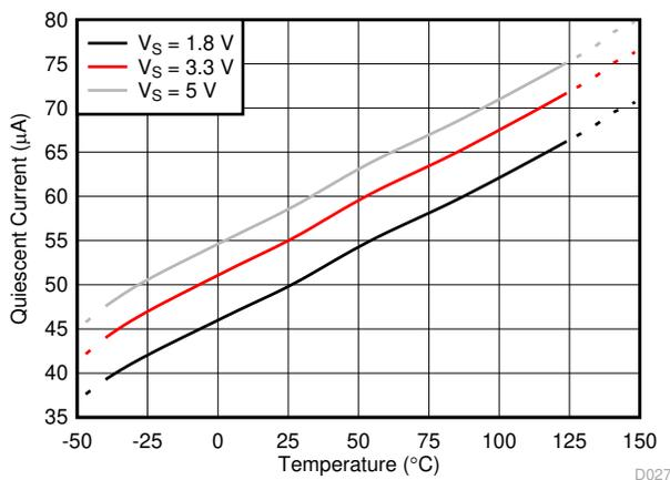
**Figure 6-17. Quiescent Current vs. Temperature (Enabled)**
