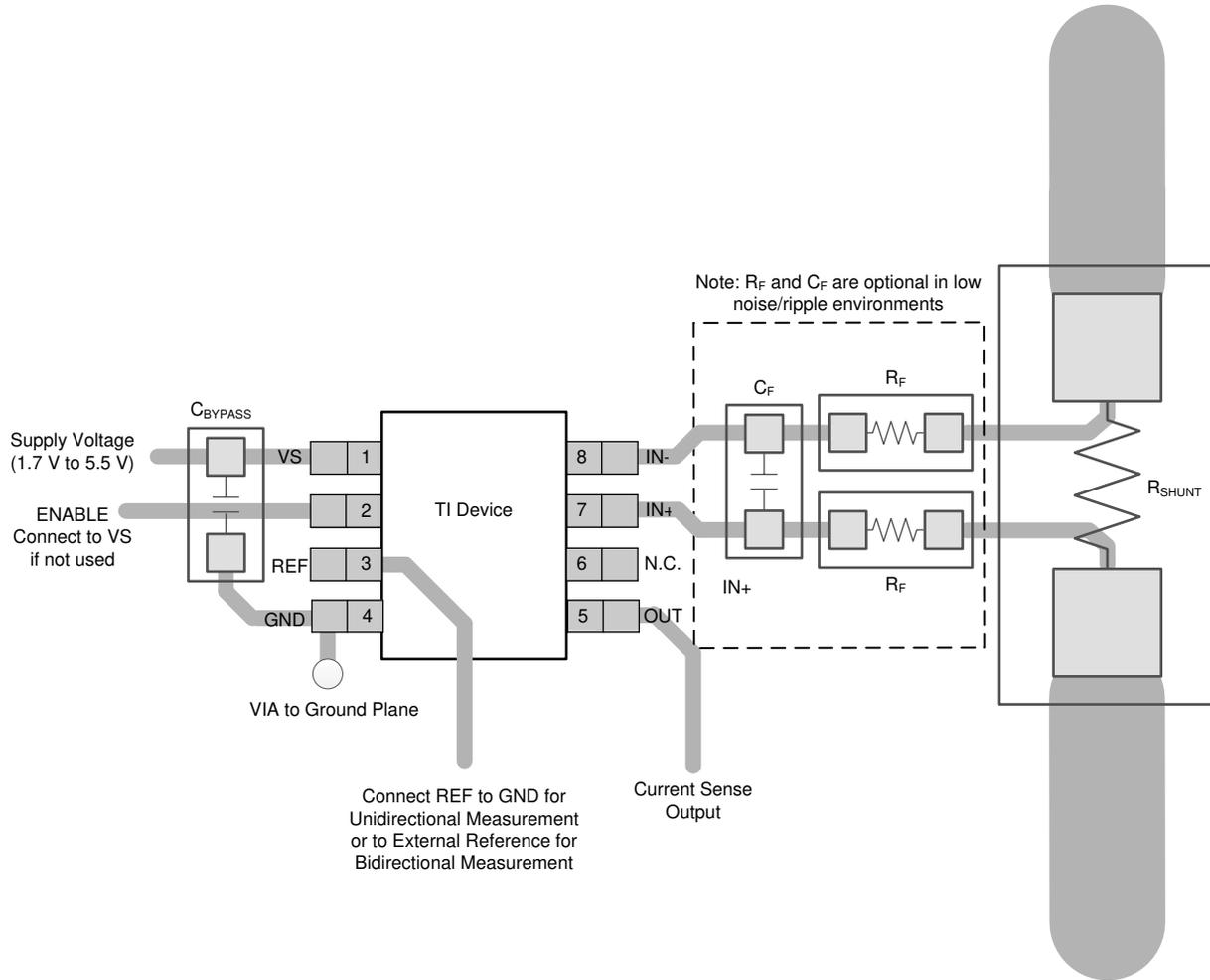
Figure 10-2. Recommended Layout for SOT23-8 (DDF) Package
