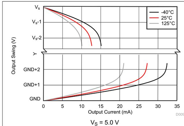
**Figure 6-13. Output Voltage Swing vs. Output Current**
