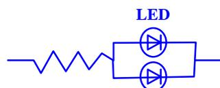
(B) The difference of brightness between LEDs could be found due to the Vf-If characteristics of LED
