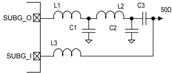
**Figure 5.8. Typical 315 MHz Band RF impedance-matching network circuit**
