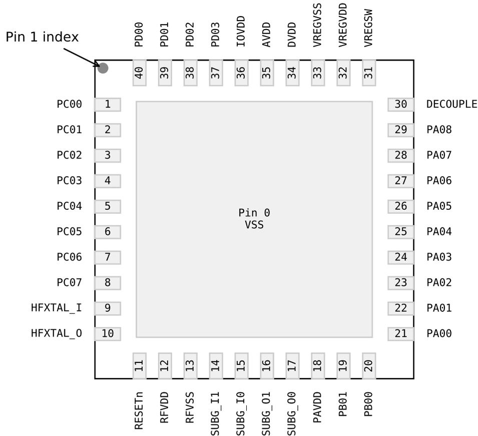
Figure 6.3. QFN40 Device Pinout
