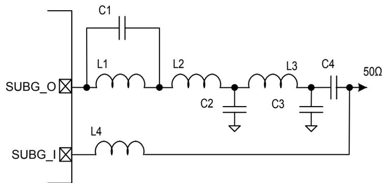
**Figure 5.5. Typical 868/915/920 MHz RF impedance-matching network circuit, +20 dBm**
