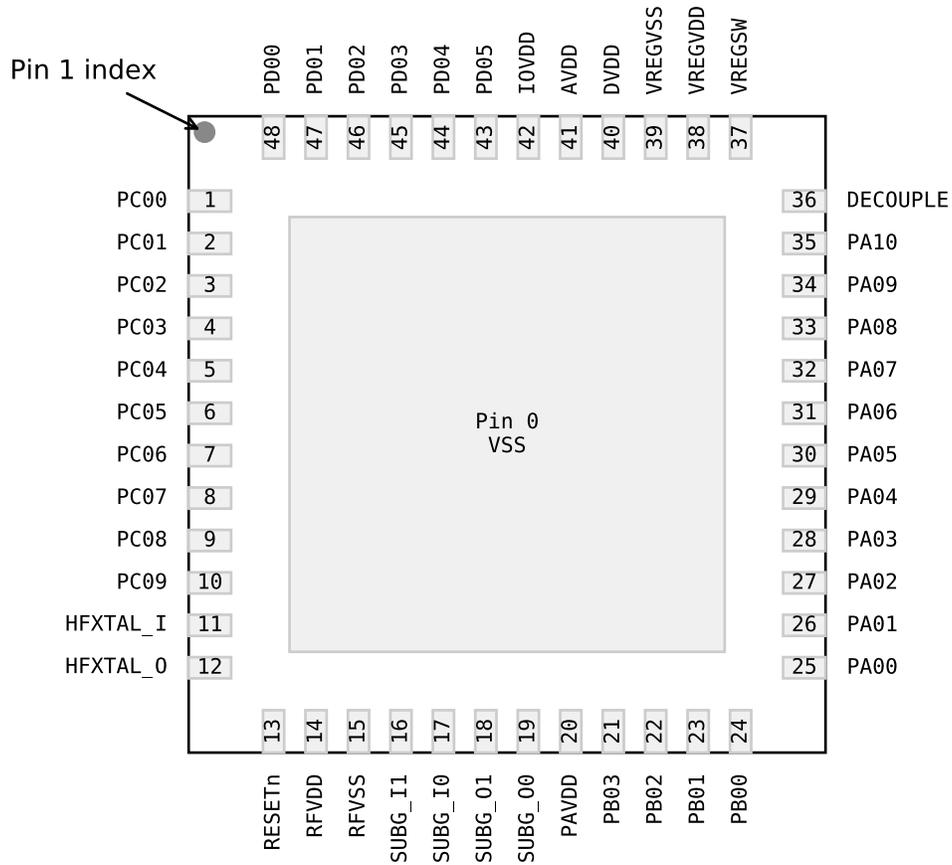
Figure 6.1. QFN48 Device Pinout
