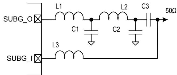
Figure 5.7. Typical 433 MHz Band RF impedance-matching network circuit
