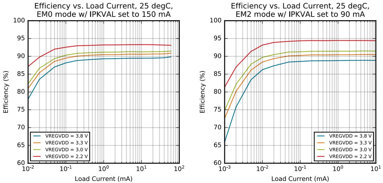
Figure 4.10. DC-DC Efficiency
