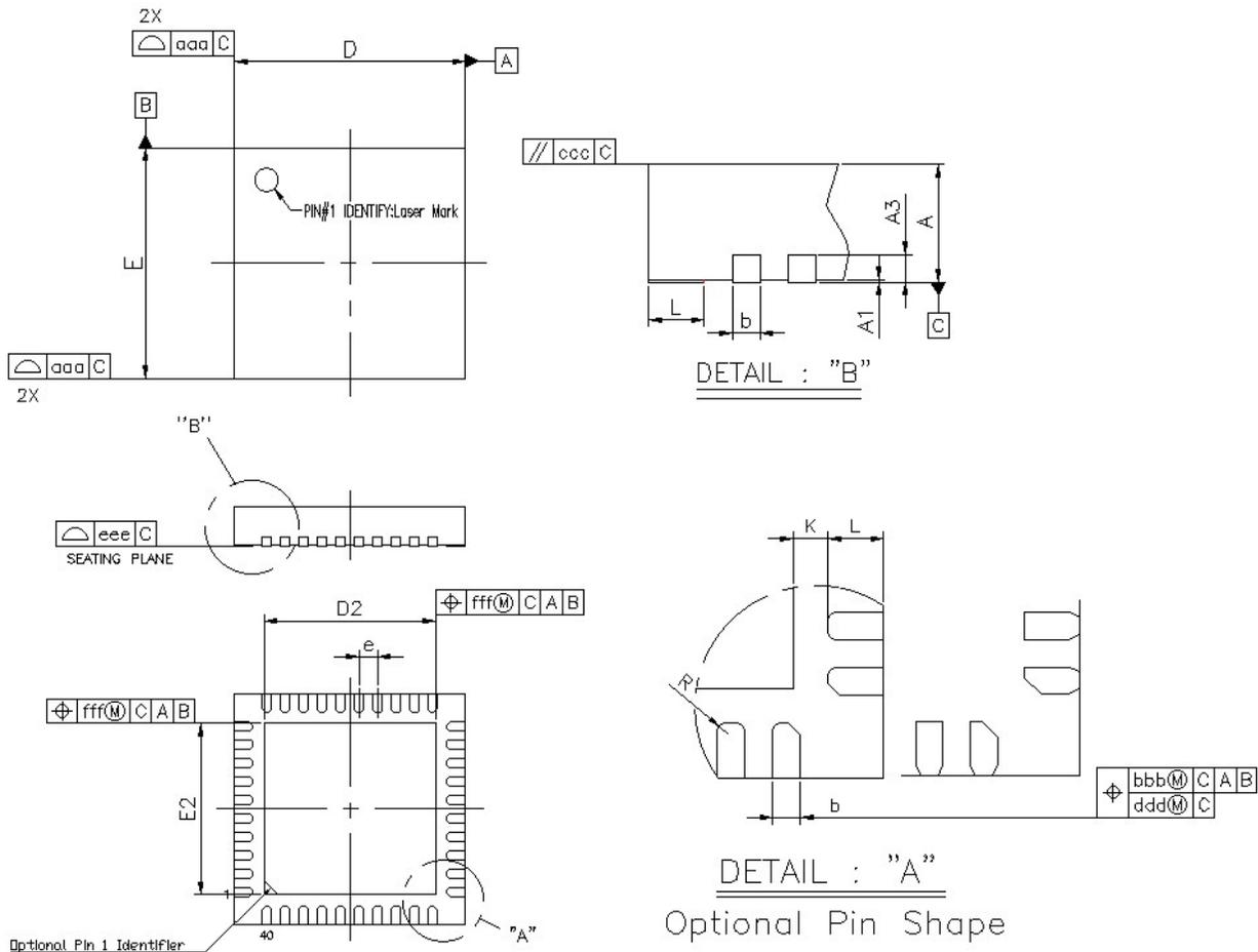
Figure 7.1. QFN40 Package Drawing
