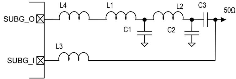
**Figure 5.6. Typical 470 MHz Band RF impedance-matching network circuit**
