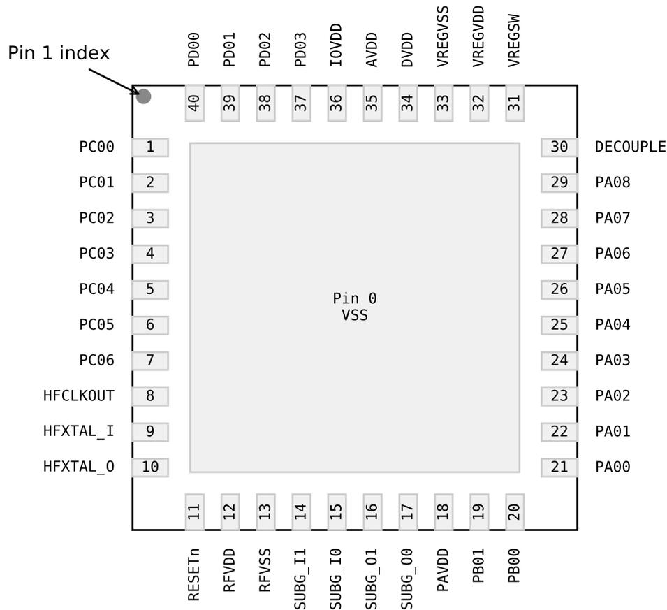
Figure 6.4. QFN40 with HFCLKOUT Device Pinout
