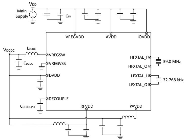
Figure 5.2. EFR32FG23 Typical Application Circuit: DCDC Configuration
