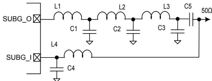
**Figure 5.9. Typical 169 MHz Band RF impedance-matching network circuit**
