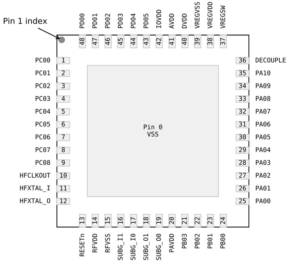
Figure 6.2. QFN48 with HFCLKOUT Device Pinout
