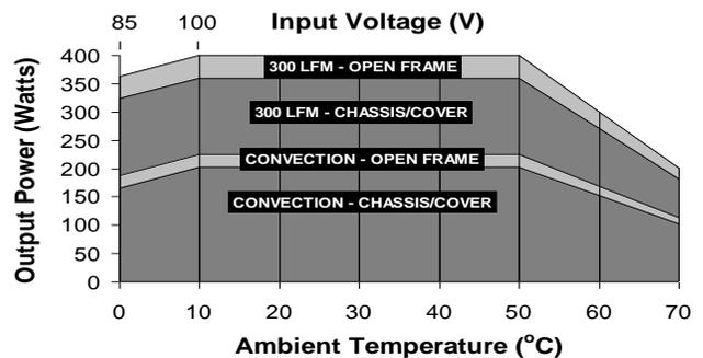
**Derating requirements** – Chart above applies to models 1003 thru 1008 only. 400W 300LFM forced air, open frame. 225W convection cooled open frame. Derate 10% with chassis and cover. Derate 2.5W<sub>OUT</sub>/1V<sub>IN</sub> below 100V<sub>IN</sub> and between 100V<sub>IN</sub> and 85V<sub>IN</sub>. Use larger of the two deratings when using chassis/cover below 100V<sub>IN</sub>. Derate output power linearly to 50% between 50° and 70°C.
