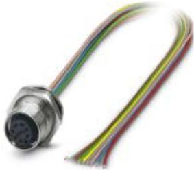
Sensor/actuator flush-type socket, 8-pos., M12 SPEEDCON, rear/screw mounting with M16 thread, with 0.5 m TPE litz wire, 8 x 0.25 mm<sup>2</sup>
