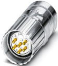
Cable connector, straight, shielded: yes, Screw locking, M23, Number of positions: 7, Type of contact: Male connector, Crimp connection, Cable diameter: 3 mm ... 14.5 mm
