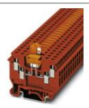
Knife disconnect terminal block, With test socket screws for insertion of test plugs, nom. voltage: 630 V, nominal current: 16 A, connection method: Screw connection, cross section: 0.2 mm² - 6 mm², AWG: 24 - 10, length: 63.5 mm, width: 6.2 mm, color: red, mounting: NS 35/7,5, NS 35/15, NS 32
