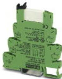
PLC-INTERFACE, consisting of DIN rail-mountable basic terminal block with spring connection and plug-in miniature relay with power contact, 1 PDT, input voltage: 120 V AC/110 V DC, UL/cUL: approved for use in Ex Zone Class I, Div. 2
