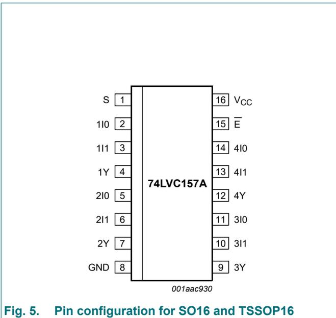
Fig. 5. Pin configuration for SO16 and TSSOP16
