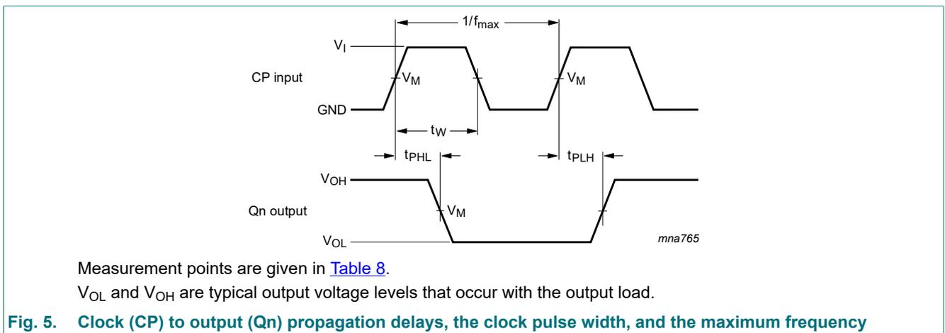
Octal D-type flip-flop with reset; positive-edge trigger
