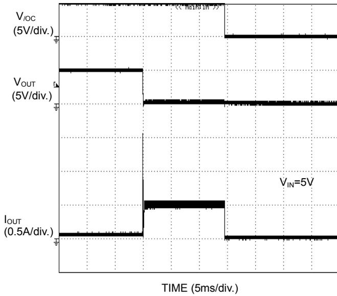
Figure 33. Over-Current Response Output Short Circuit at Enable
