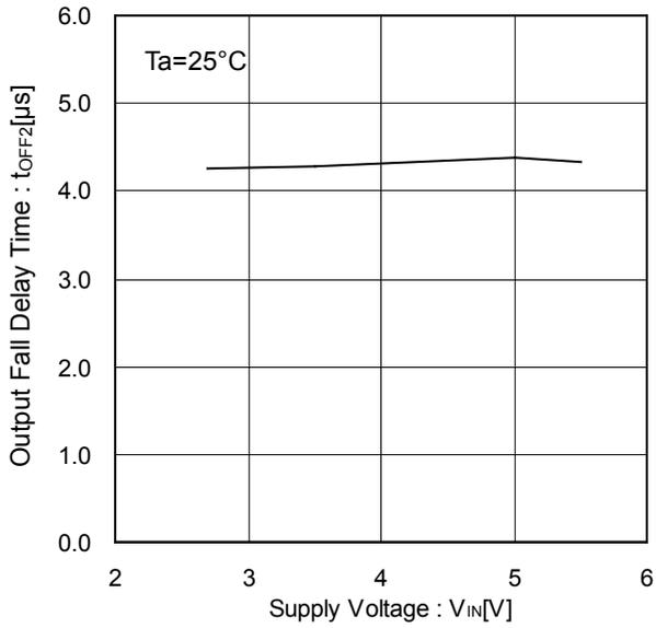
Figure 23. Output Fall Delay Time vs Supply Voltage
