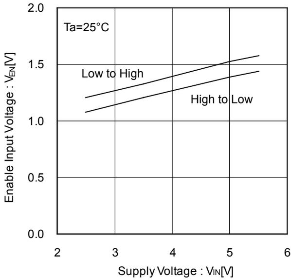
Figure 7. EN Input Voltage vs Supply Voltage
