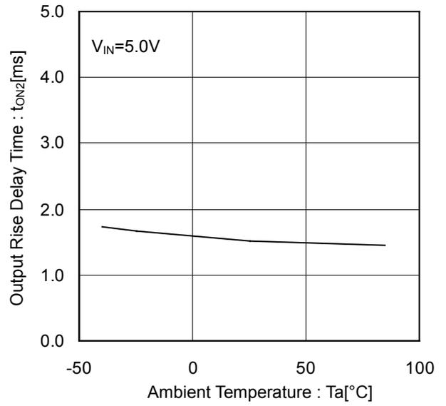
Figure 20. Output Rise Delay Time vs Ambient Temperature
