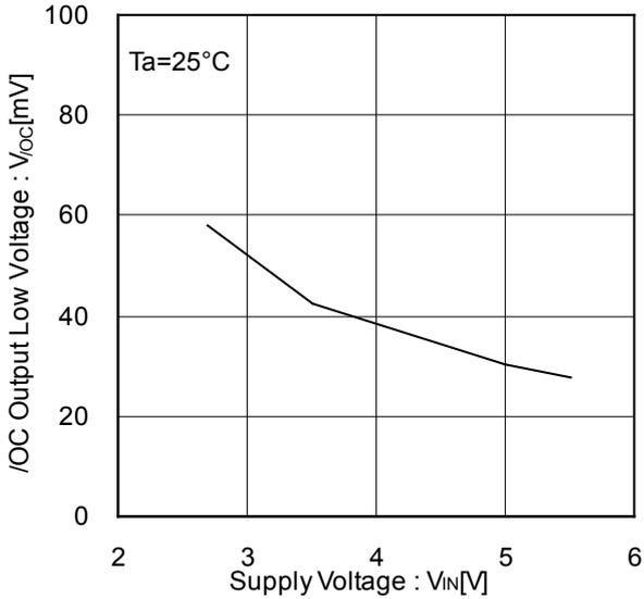
Figure 13. /OC Output Low Voltage vs Supply Voltage
