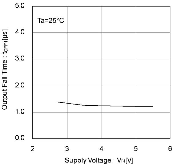
Figure 21. Output Fall Time vs Supply Voltage
