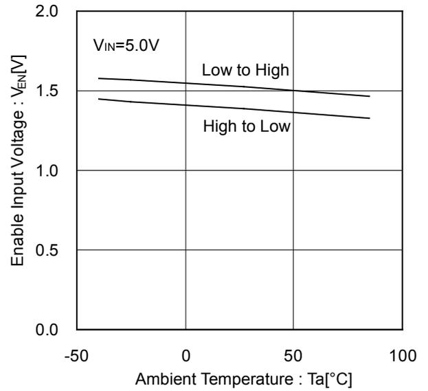
Figure 8. EN Input Voltage vs Ambient Temperature
