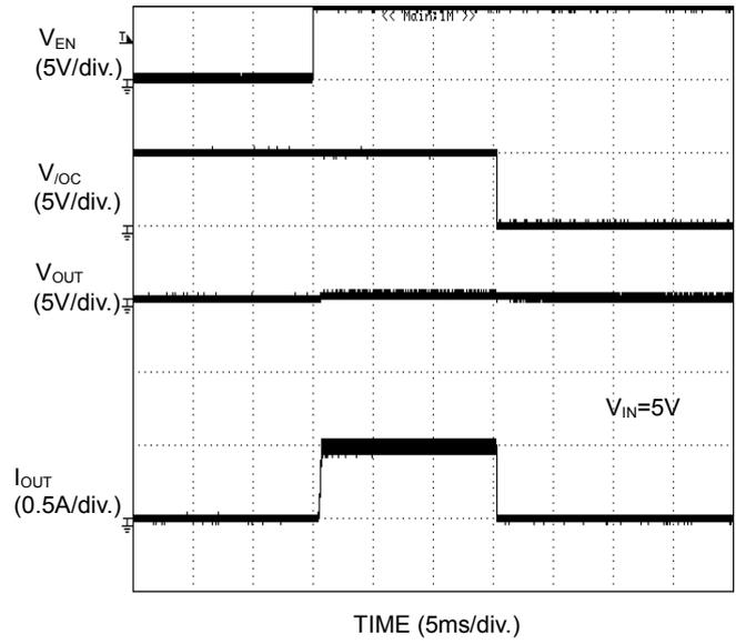
Figure 32. Over-Current Response Enable to Short Circuit
