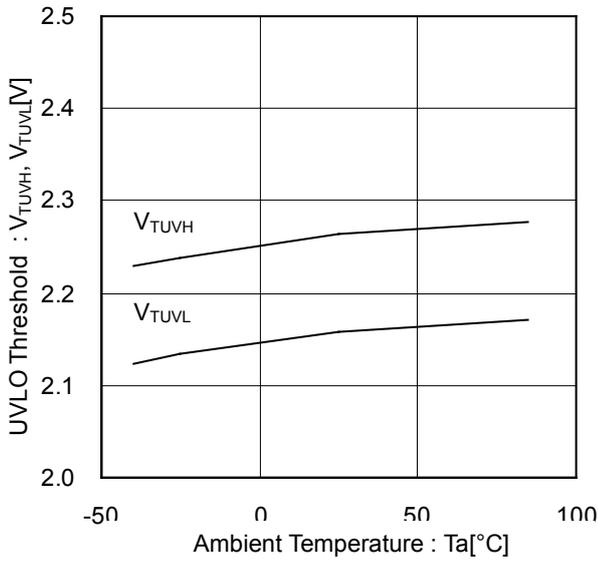
Figure 15. UVLO Threshold Voltage vs Ambient Temperature
