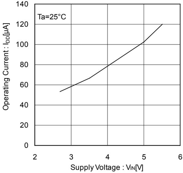
Figure 3. Operating Current vs Supply Voltage (EN Enable)
