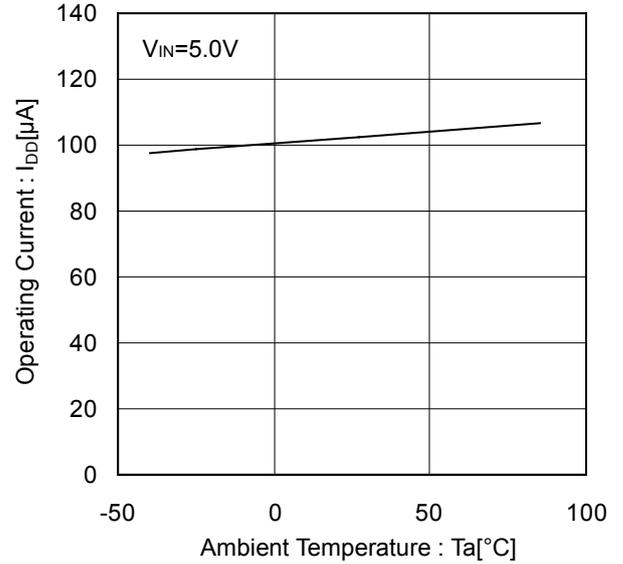
Figure 4. Operating Current vs Ambient Temperature (EN Enable)
