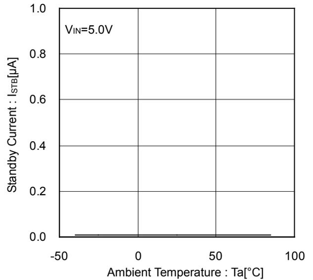
Figure 6. Standby Current vs Ambient Temperature (EN Disable)
