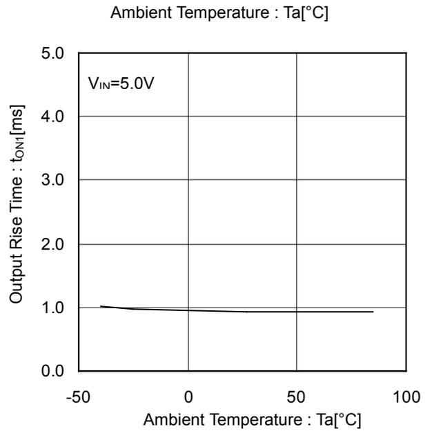
Figure 18. Output Rise Time vs Ambient Temperature
