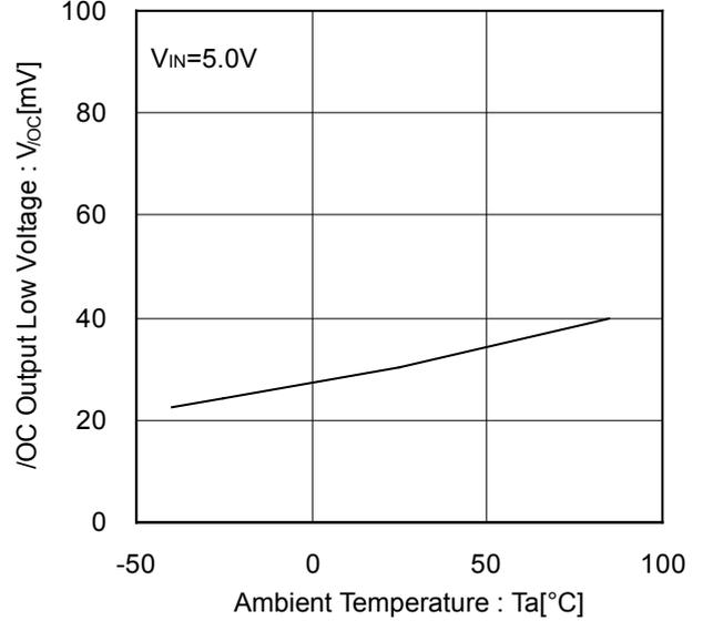
Figure 14. /OC Output Low Voltage vs Ambient Temperature
