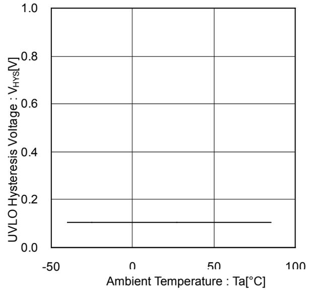
Figure 16. UVLO Hysteresis Voltage vs Ambient Temperature
