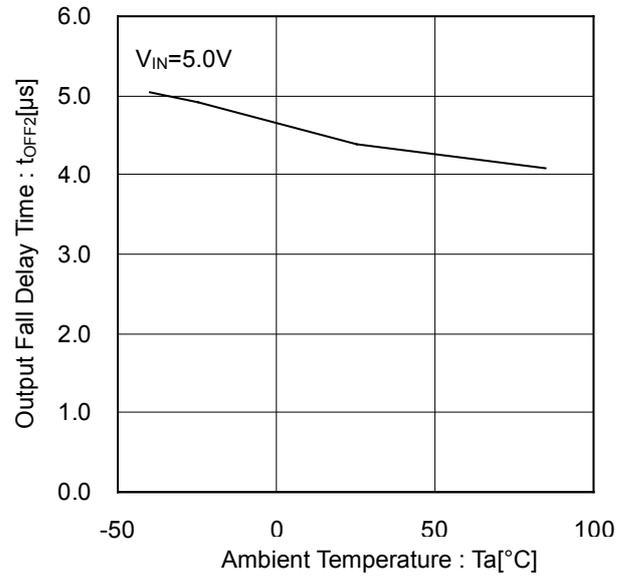
Figure 24. Output Fall Delay Time vs Ambient Temperature
