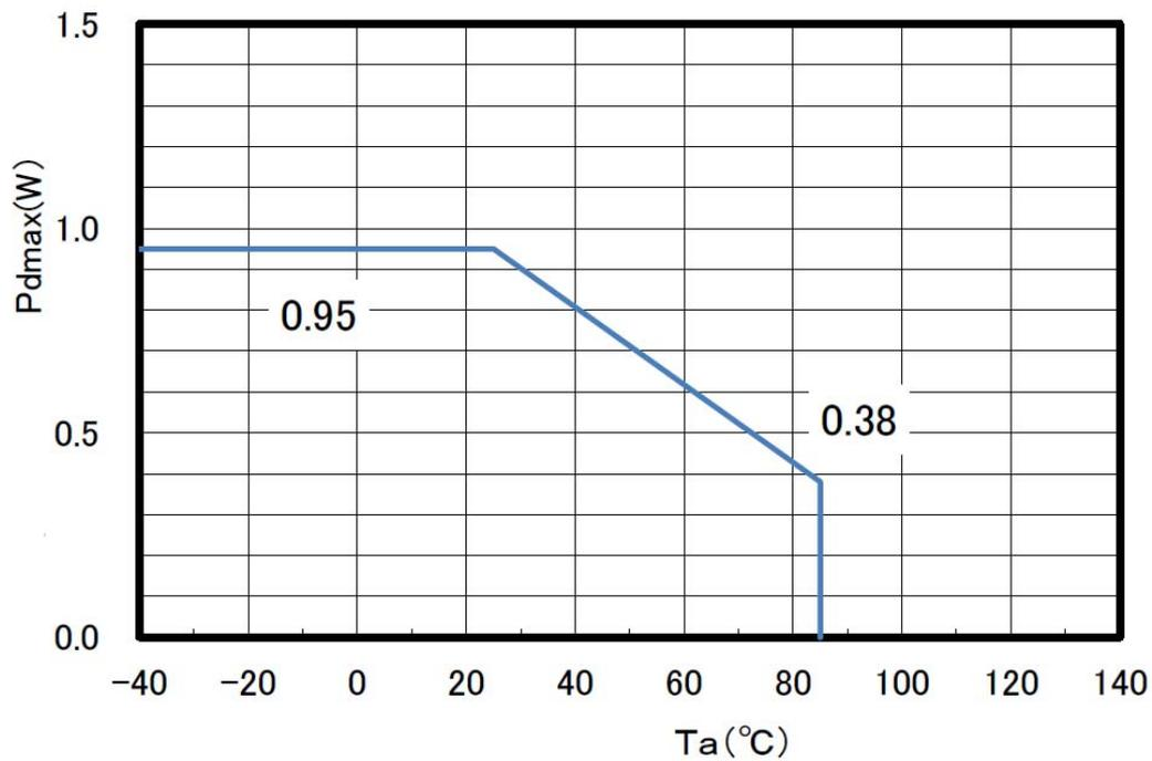
Mounted on a specified board : 70mm×70mm×1.6mm (4 layer glass epoxy)
