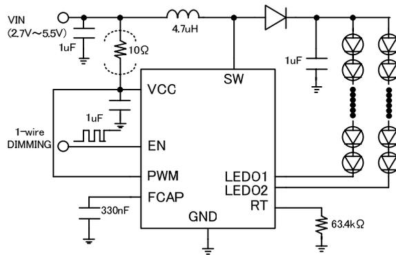
1-wire dimming mode and PWM dimming mode (CABC)
