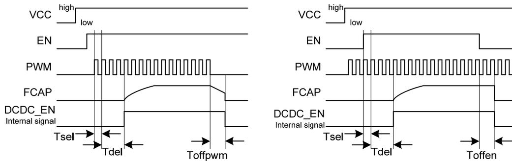
Fig6. Start up and shutdown diagram (**PWM MODE**)
