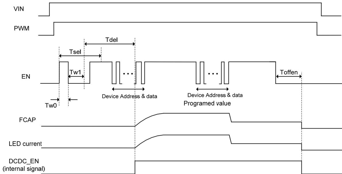
Fig3. Start up and shutdown diagram (**DIGITAL MODE**)
