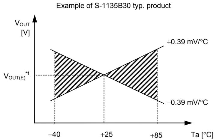
\*1.  $V_{OUT(E)}$  is the value of the output voltage measured at  $T_a = +25^{\circ}\text{C}$ .
