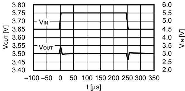
2. Transient Response Characteristics of Load (Ta = 25°C)
