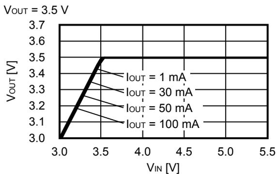
**3. Dropout Voltage vs. Output Current**
