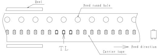
Those with one electrode terminal on the feed hole side·····TL
