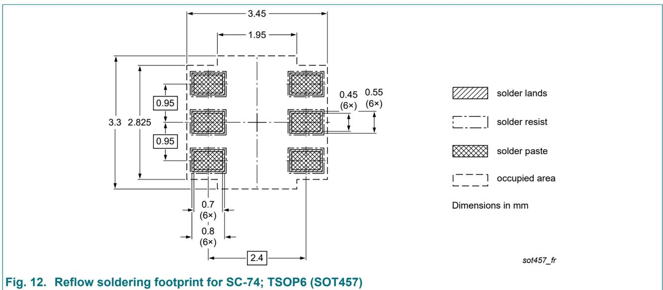
Fig. 12. Reflow soldering footprint for SC-74; TSOP6 (SOT457)
