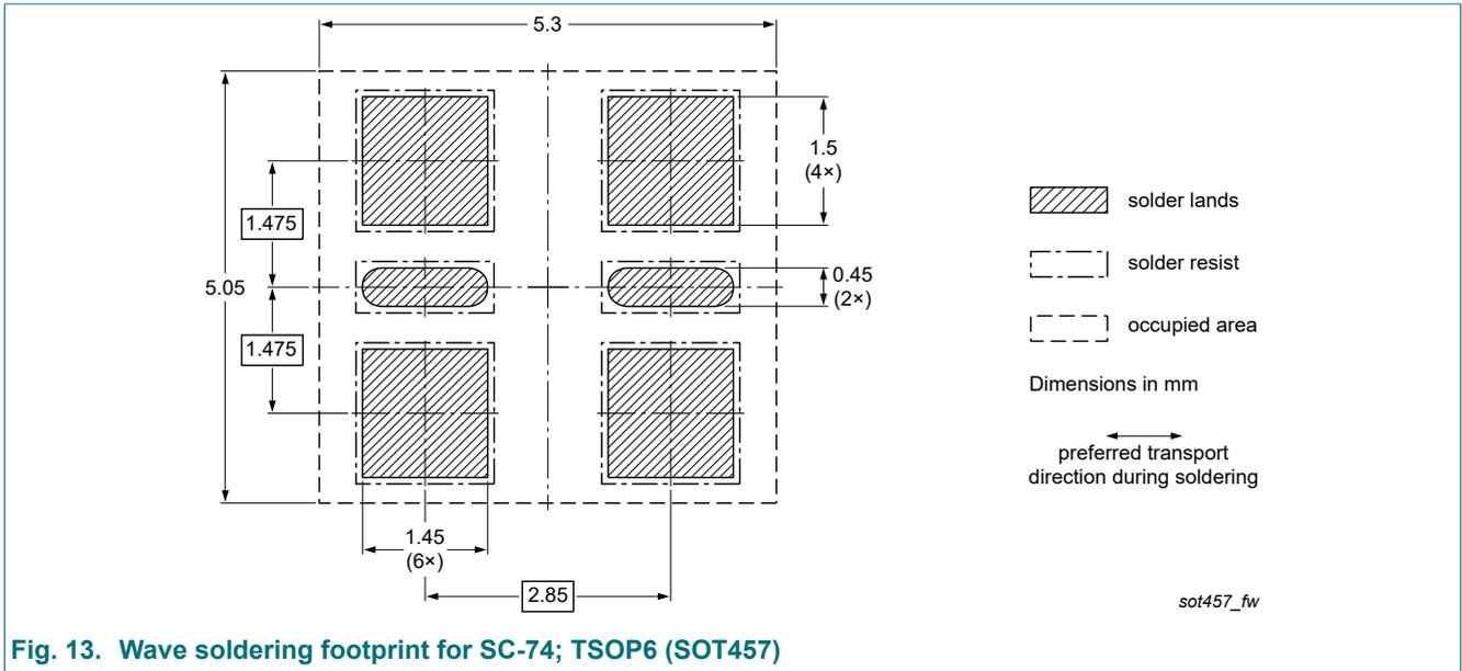
Fig. 13. Wave soldering footprint for SC-74; TSOP6 (SOT457)
