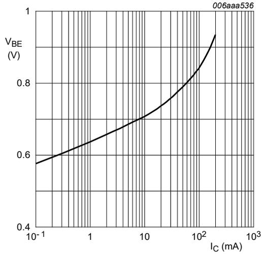
$V_{CE} = 5$  V;  $T_{amb} = 25$  °C
