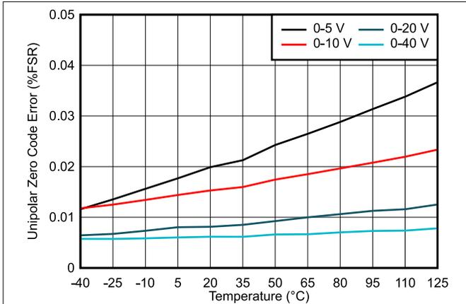
Figure 7-21. Unipolar Zero Code Error vs Temperature
