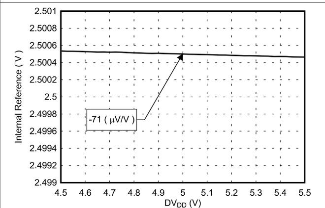
**Figure 7-44. Internal Reference Voltage vs Supply Voltage**
