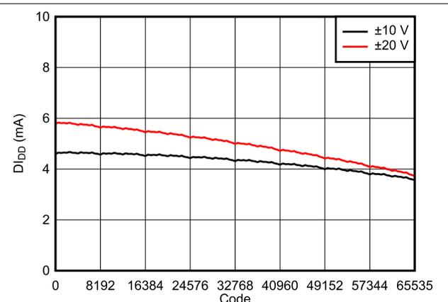
Figure 7-26. Supply Current ( $DI_{DD}$ ) vs Digital Input Code
