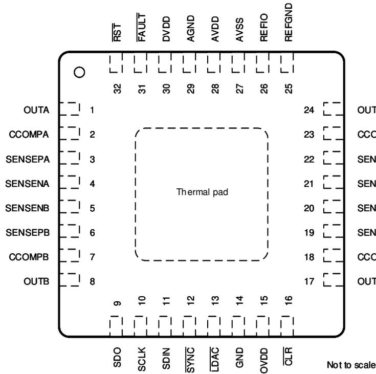
Figure 6-1. RHB (32-pin VQFN) Package, Top View
