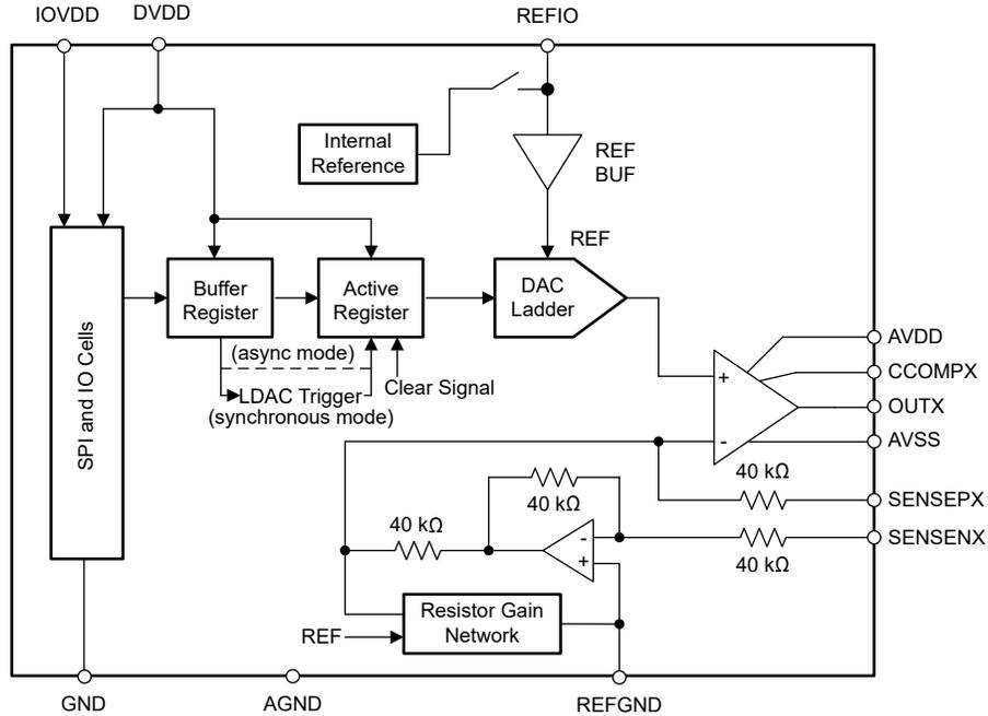
Figure 8-1. Device Architecture
