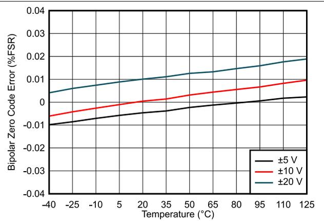
Figure 7-22. Bipolar Zero Code Error vs Temperature
