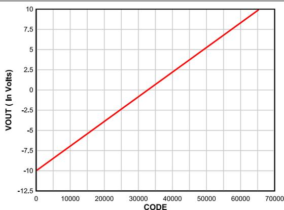
Figure 9-2. DAC Code Sweep From  $-10$  V to  $+10$  V
