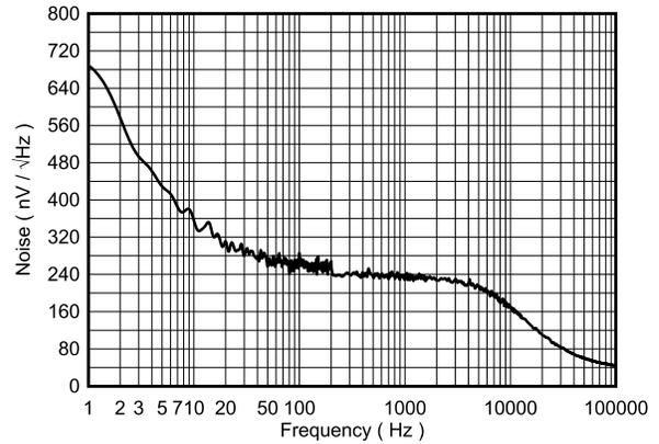
**Figure 7-46. Internal Reference Noise Density vs Frequency**
