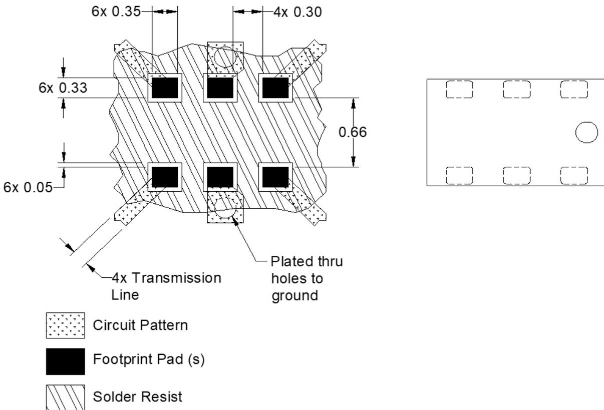
Dimensions are in Millimeters
