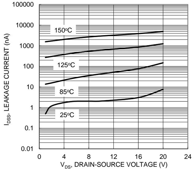
Figure 10. Typical Drain-Source Leakage Current vs. Voltage
