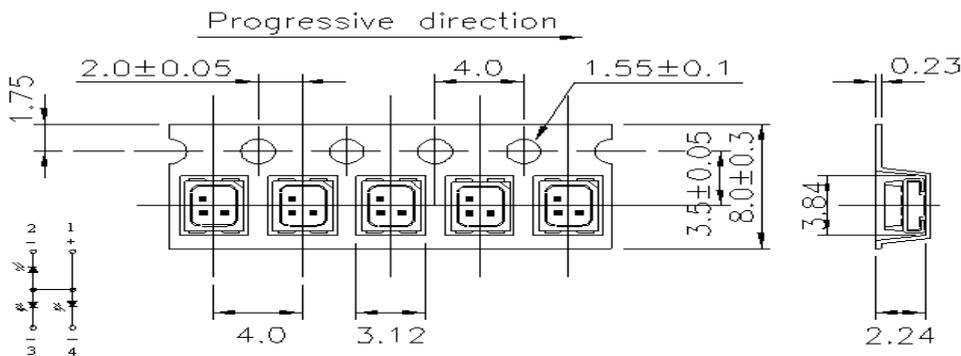
Note: Tolerances unless mentioned  $\pm 0.1$ mm. Unit = mm
