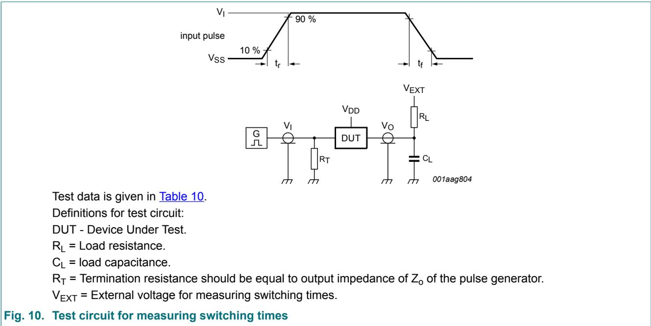
Fig. 10. Test circuit for measuring switching times
