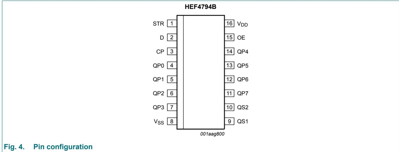
Fig. 4. Pin configuration
