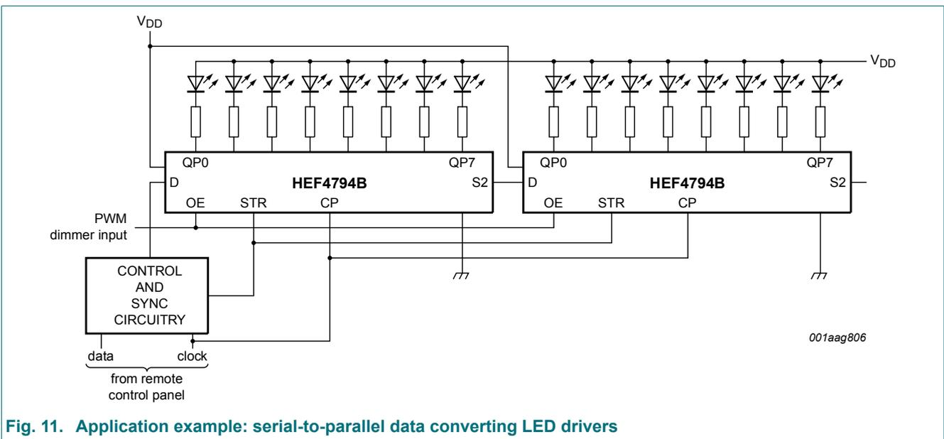
Fig. 11. Application example: serial-to-parallel data converting LED drivers
