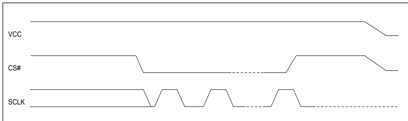
**Figure 48. Power-up Timing**
