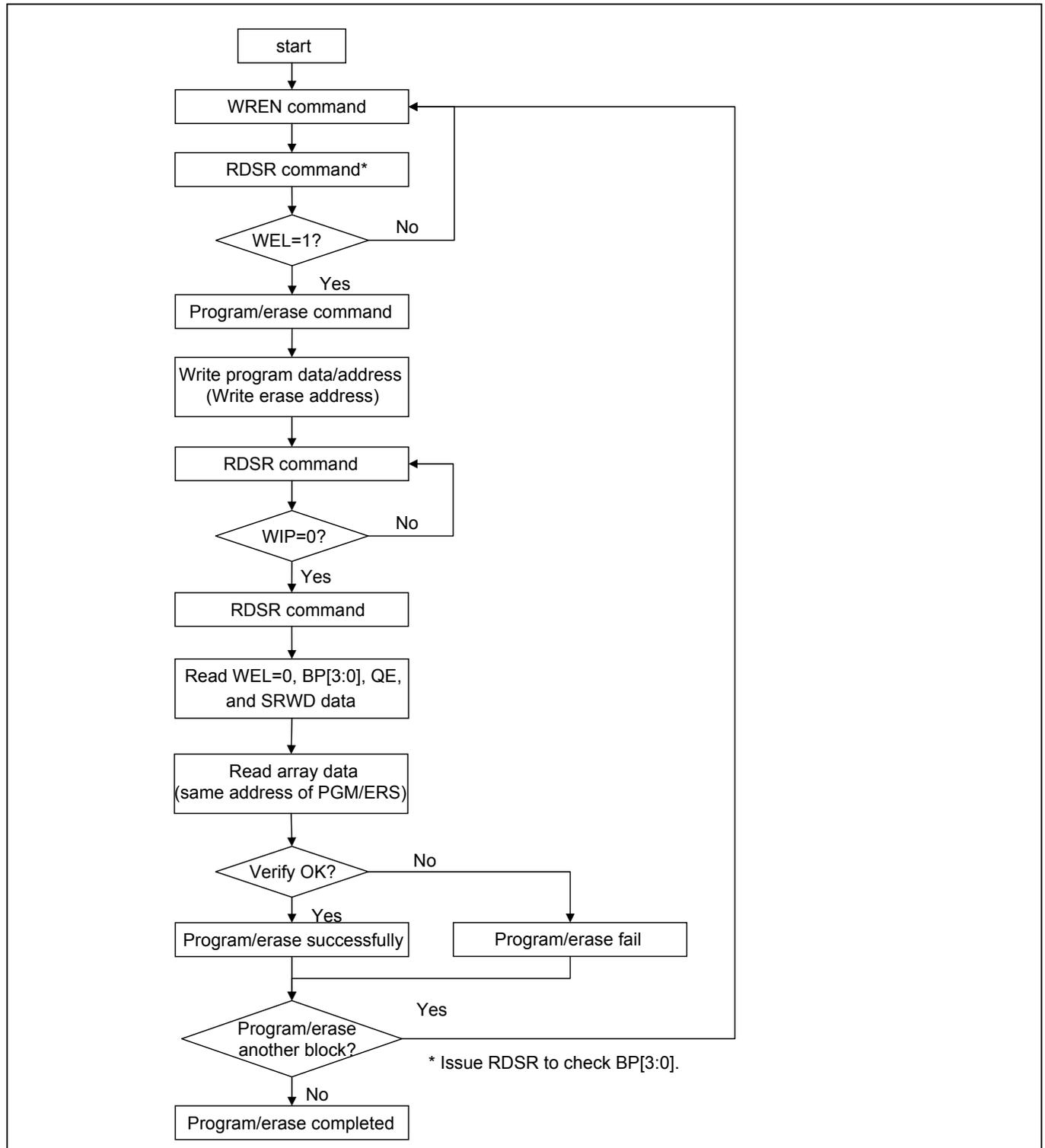
Figure 13. Program/Erase flow without read array data (read P\_FAIL/E\_FAIL flag)
