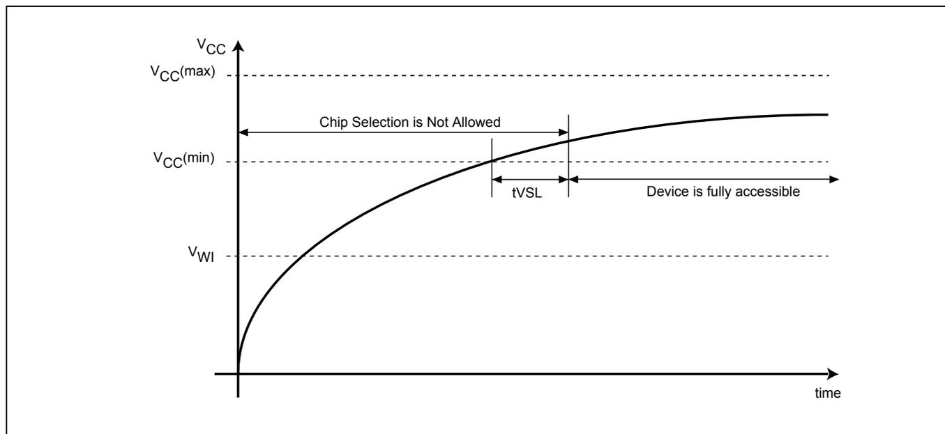
**Figure 49. Power Up/Down and Voltage Drop**
