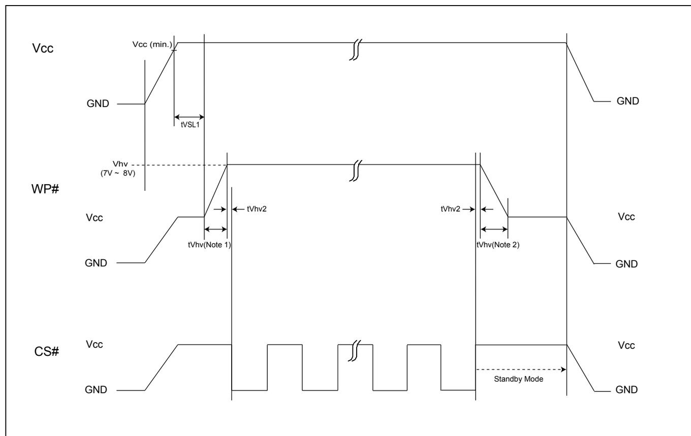
**Note 1:** Please note that the CS# can only go low after  $tVSL1+tVhv +tVhv2$  timing during High Voltage Operation.
