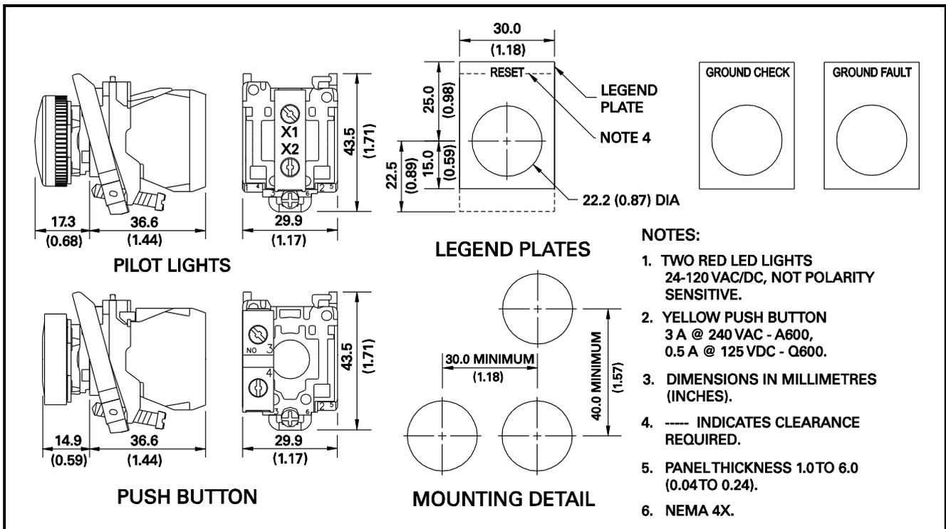
FIGURE 9. RK-132 Remote Indication and Reset Kit.
