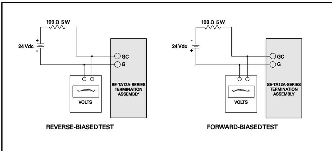
FIGURE 17. Termination-Assembly-Test Circuits.
