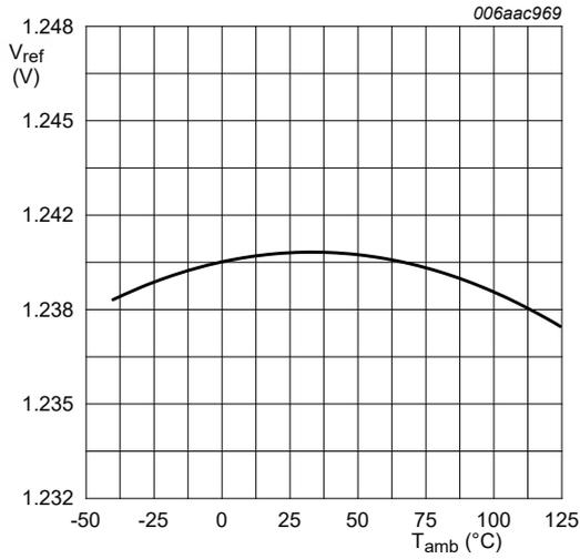
$I_K = 10 \text{ mA}; V_{KA} = V_{ref}$
