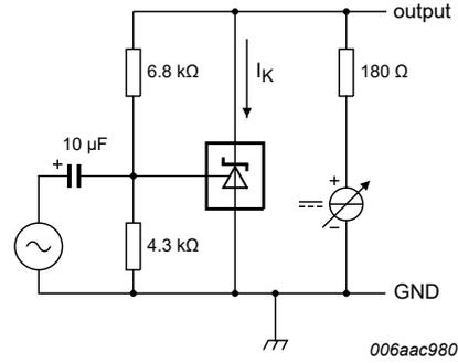
$I_K = 10 \text{ mA}; T_{\text{amb}} = 25 \text{ }^\circ\text{C}$
