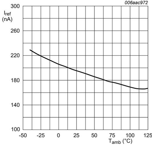
V<sub>KA</sub> = 1.24 V; I<sub>K</sub> = 10 mA; R<sub>1</sub> = 10 kΩ; R<sub>2</sub> = open
