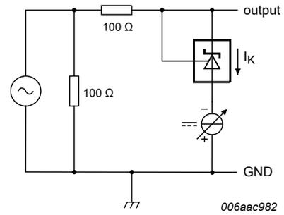
$I_K = 10 \text{ mA}; T_{\text{amb}} = 25 \text{ }^\circ\text{C}$
