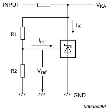
$$V_{KA} = V_{ref} \times (1 + R1/R2) + I_{ref} \times R1$$
