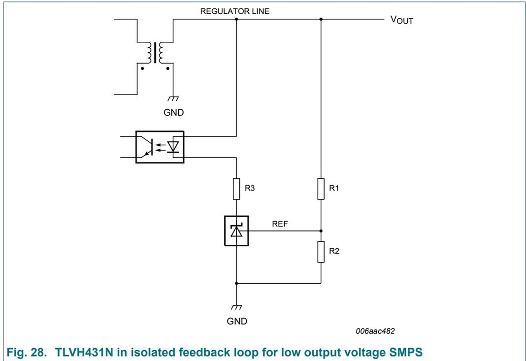
Fig. 28. TLVH431N in isolated feedback loop for low output voltage SMPS
