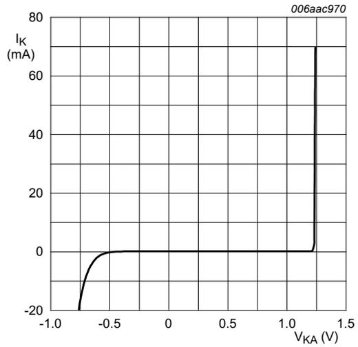
$V_{KA} = V_{ref}; T_{amb} = 25 \text{ °C}$
