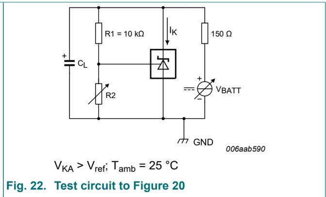
Figures 20, 21 and 22 show the stability boundaries and test circuits for the worst case conditions with a load capacitance mounted as close as possible to the device. The required load capacitance for stable operation varies depending on the operating temperature and capacitor Equivalent Series Resistance (ESR). Verify that the application circuit is stable over the anticipated operating current and temperature ranges.
