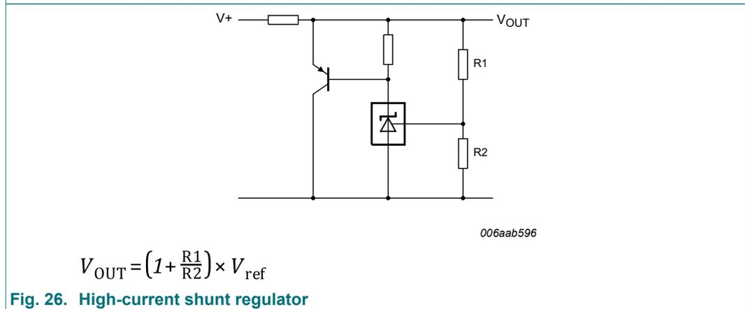
Fig. 26. High-current shunt regulator
