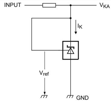
$I_K = 10 \text{ mA}; V_{KA} = V_{ref}$
