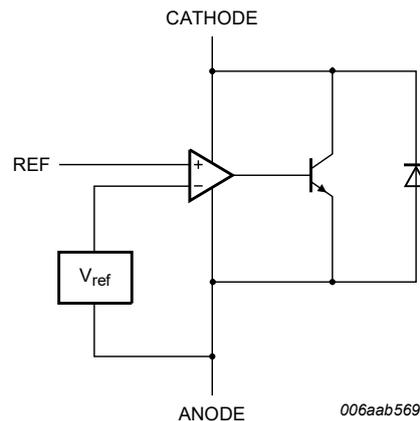
Fig. 1. Functional diagram
