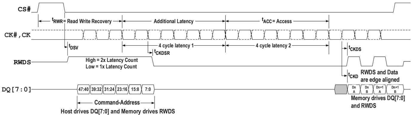
Figure 30 - Read Timing Diagram — With Additional Latency
