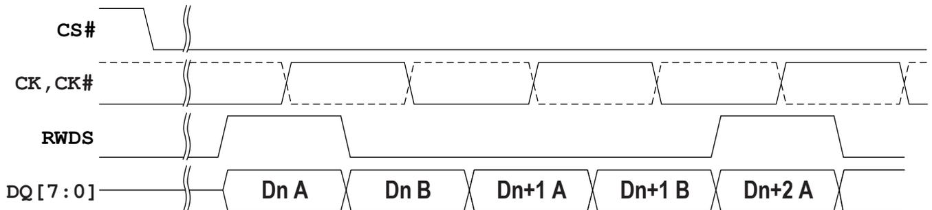
**Figure 7 - Data Placement during a Write Transaction**
