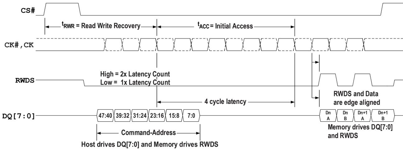
**Figure 9 - Read Transaction without Additional Initial Latency**
