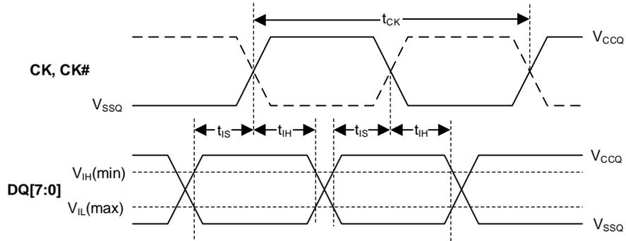
Figure 26 – DDR Input Timing Reference Levels
