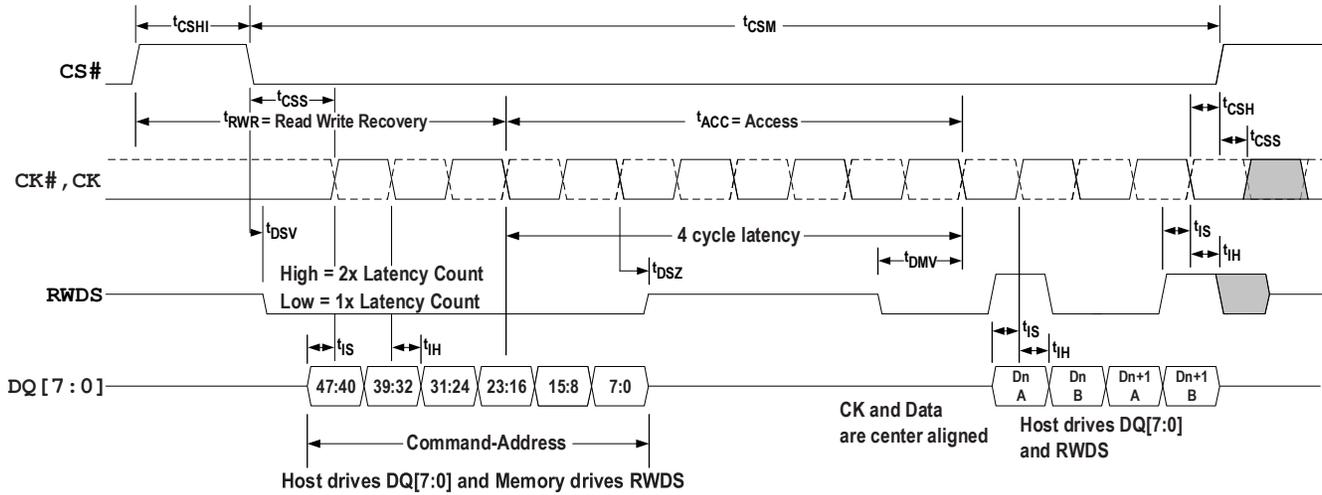
Figure 32 - Write Timing Diagram — No Additional Latency
