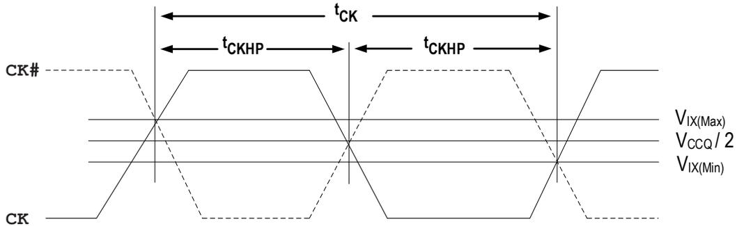
Figure 28 - Clock Characteristics
