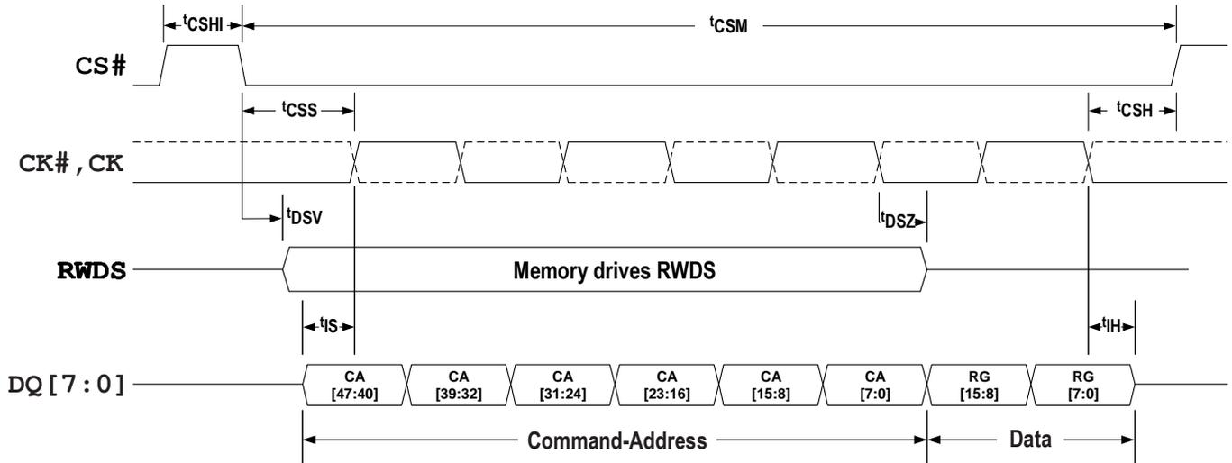
Figure 34 - Write Operation without Initial Latency (Register Write)
