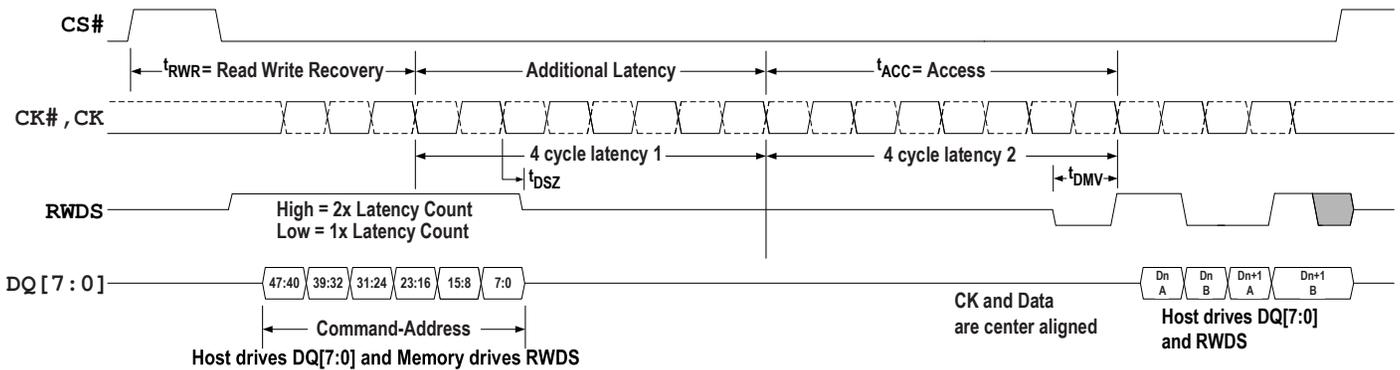
Figure 33 - Write Timing Diagram — With Additional Latency
