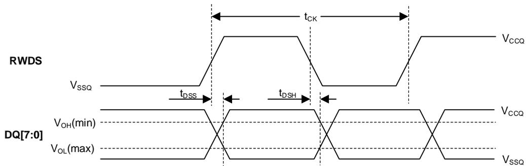
Figure 27 – DDR Output Timing Reference Levels
