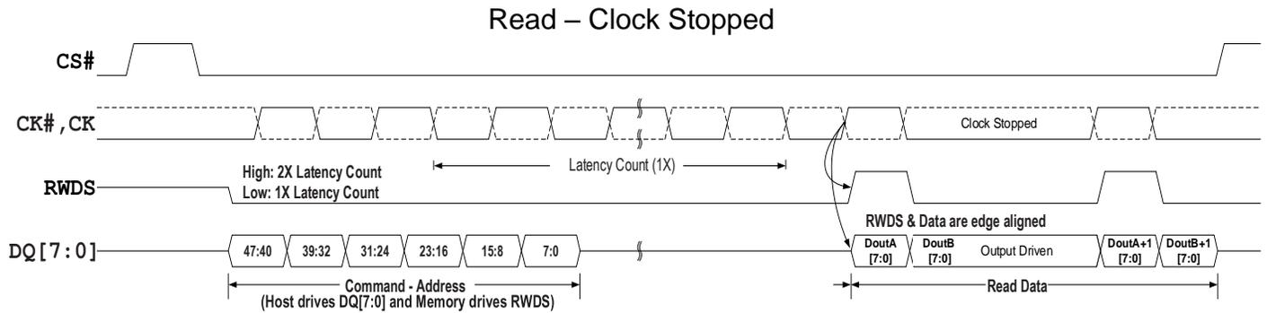
Figure 13 - Active Clock Stop during Read Transaction (DDR)
