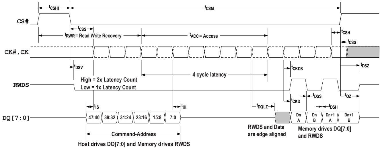
Figure 29 - Read Timing Diagram — No Additional Latency Required
