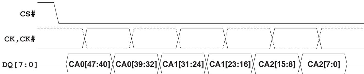
**Figure 5 - Command-Address (CA) Sequence**
