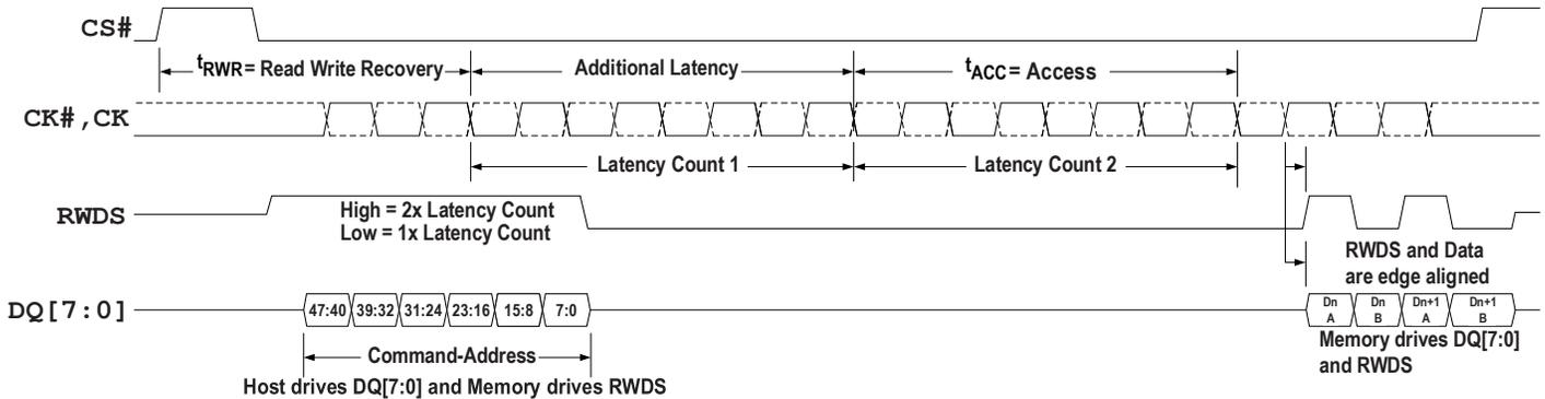
**Figure 2 - Read Transaction, Additional Latency Count**
