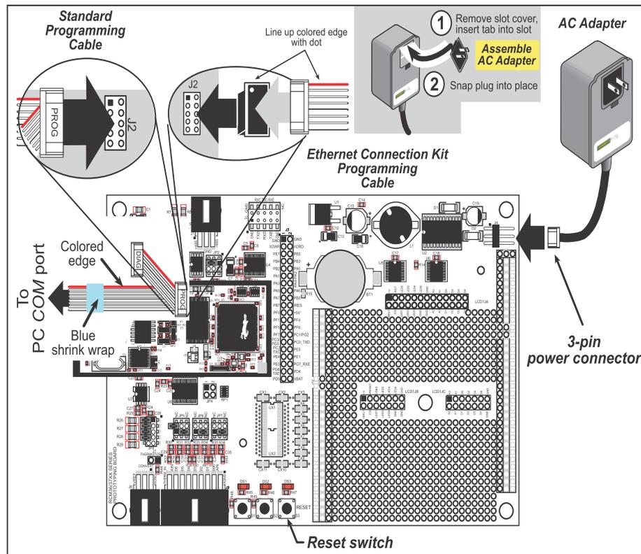
**Figure 3. Connect Programming Cable and Power Supply**
