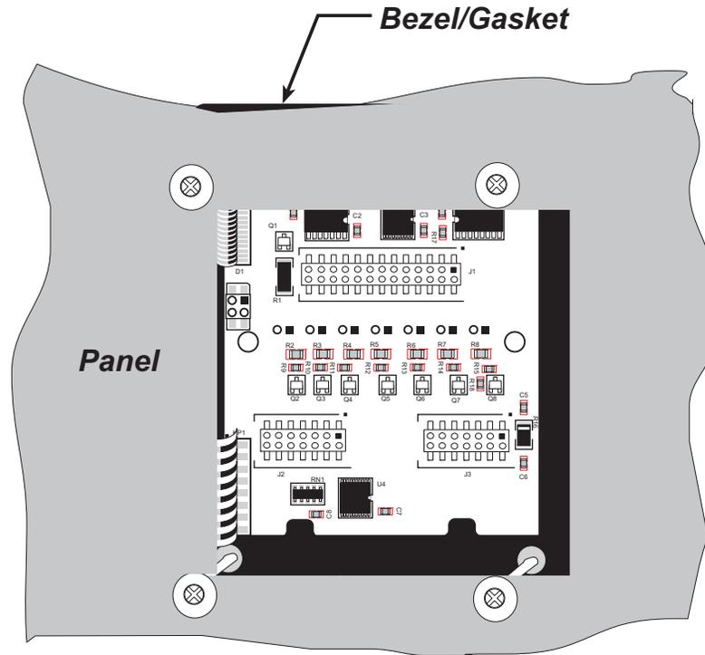
**Figure C-10. LCD/Keypad Module Mounted in Panel (rear view)**
