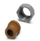
Half screw connection Pg21, made of plastic, consisting of rubber seal with one elongated hole and one pressure screw, for type 2 - 4 housings, cable diameter: 20 x 7 mm
