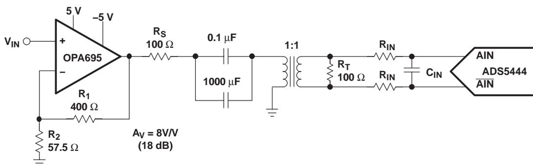
**Figure 14. Using the OPA695 with the ADS5444**
