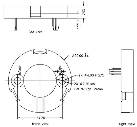
**CAUTION:** For optimal performance, base plate and plastic housing assembly are designed for a ONE time assembly process only. Removal and re-assembly process should be avoided due to the potential weakness of the latch after re-assembly.
