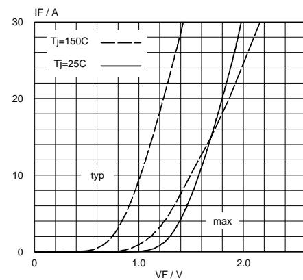
Fig.13. Damper forward characteristic  $I_F = f(V_F)$ ; parameter  $T_j$
