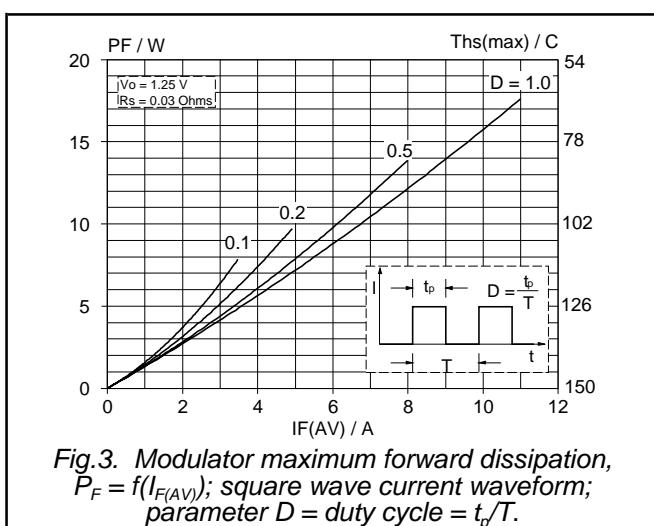
Fig.3. Modulator maximum forward dissipation,
