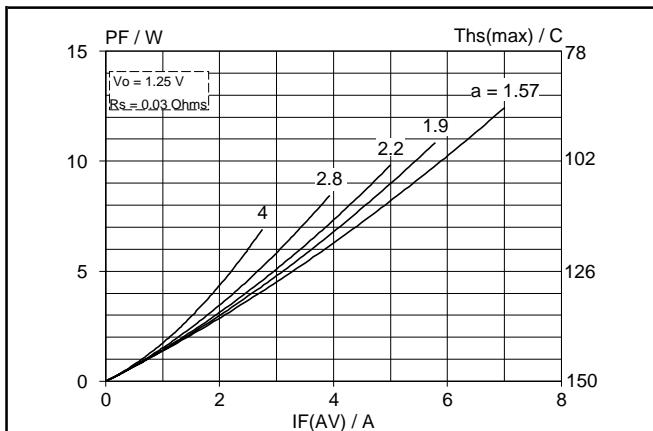
Fig.4. Modulator maximum forward dissipation,
