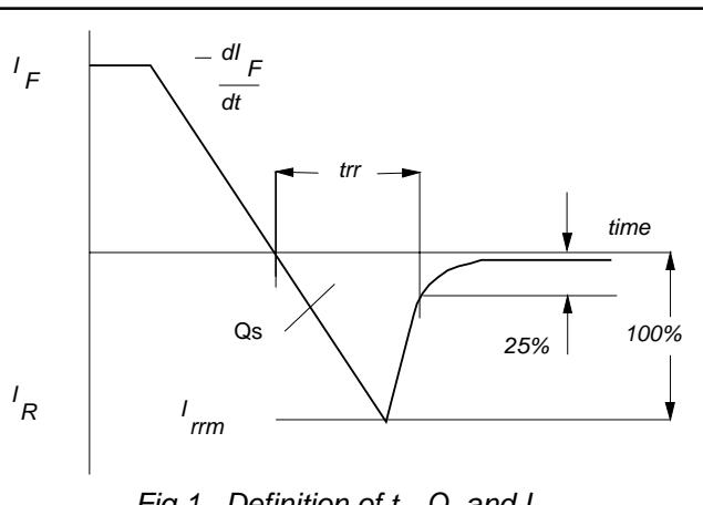
Fig.1. Definition of  $t_{rr}$ ,  $Q_s$  and  $I_{rrm}$
