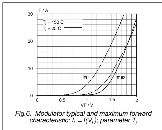
Fig.6. Modulator typical and maximum forward
