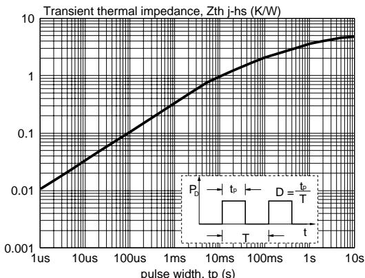
Fig.12. Damper transient thermal impedance  $Z_{th} = f(t_p)$
