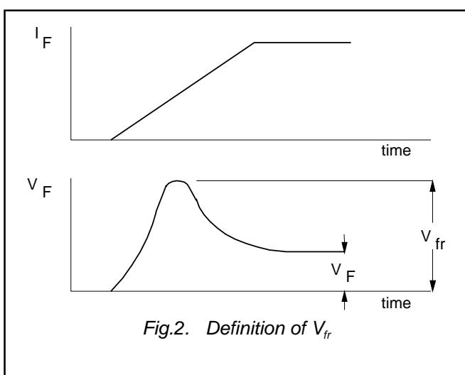
Fig.2. Definition of  $V_{fr}$
