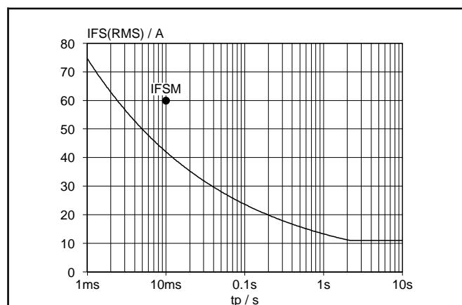
Fig.5. Modulator maximum non-repetitive rms forward current,  $I_F = f(t_p)$ ; sinusoidal current waveform;
