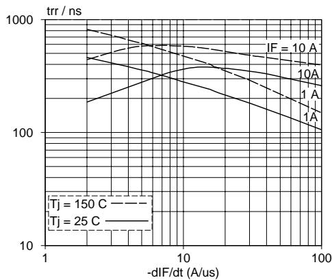
Fig.8. Modulator maximum  $t_{rr}$  measured to 25% of  $I_{rrm}$ ;  $T_j=25^\circ\text{C}$  and  $150^\circ\text{C}$
