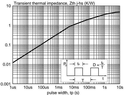
Fig.10. Modulator transient thermal impedance  $Z_{th} = f(t_p)$
