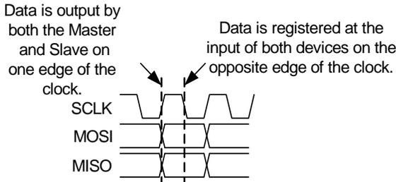
A device can be a master or slave. A master outputs clock and data to the slave device and inputs slave data. A slave device inputs clock and data from the master device and outputs data for input to the master. Together, the master and slave are essentially a circular Shift register, where the master generates the clocking and initiates data transfers.
