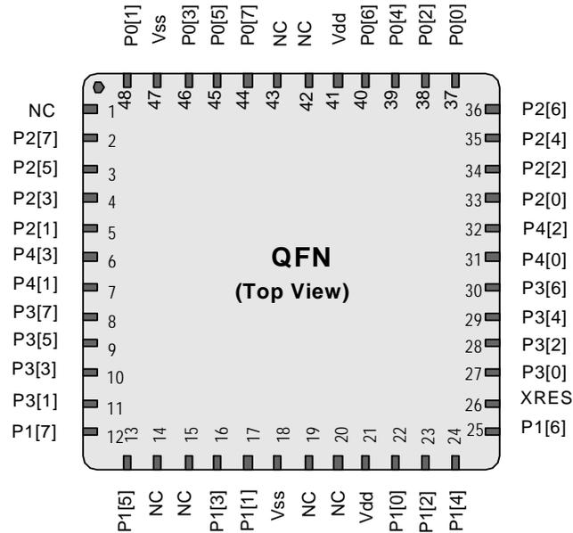
Table 3. 48-Pin Part Pinout (QFN)
