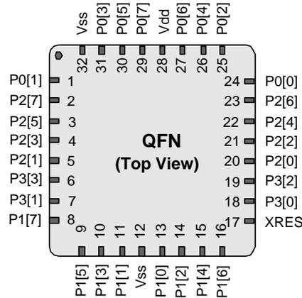
Table 2. 32-Pin Part Pinout (QFN)
