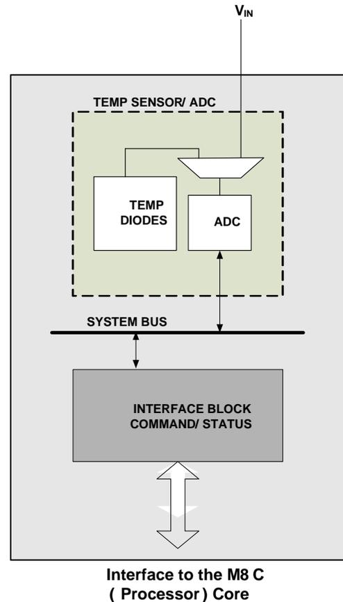
The ADC User Module contains an integrator block and one comparator with positive and negative input set by the MUXes. The input to the integrator stage comes from the Analog Global Input Mux or the temperature sensor with an input voltage range of 0 V to 1.3 V, where 1.3 V is 72% of full scale.
