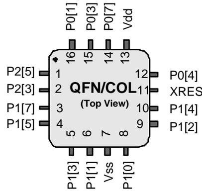
Table 1. 16-Pin Part Pinout (QFN)
