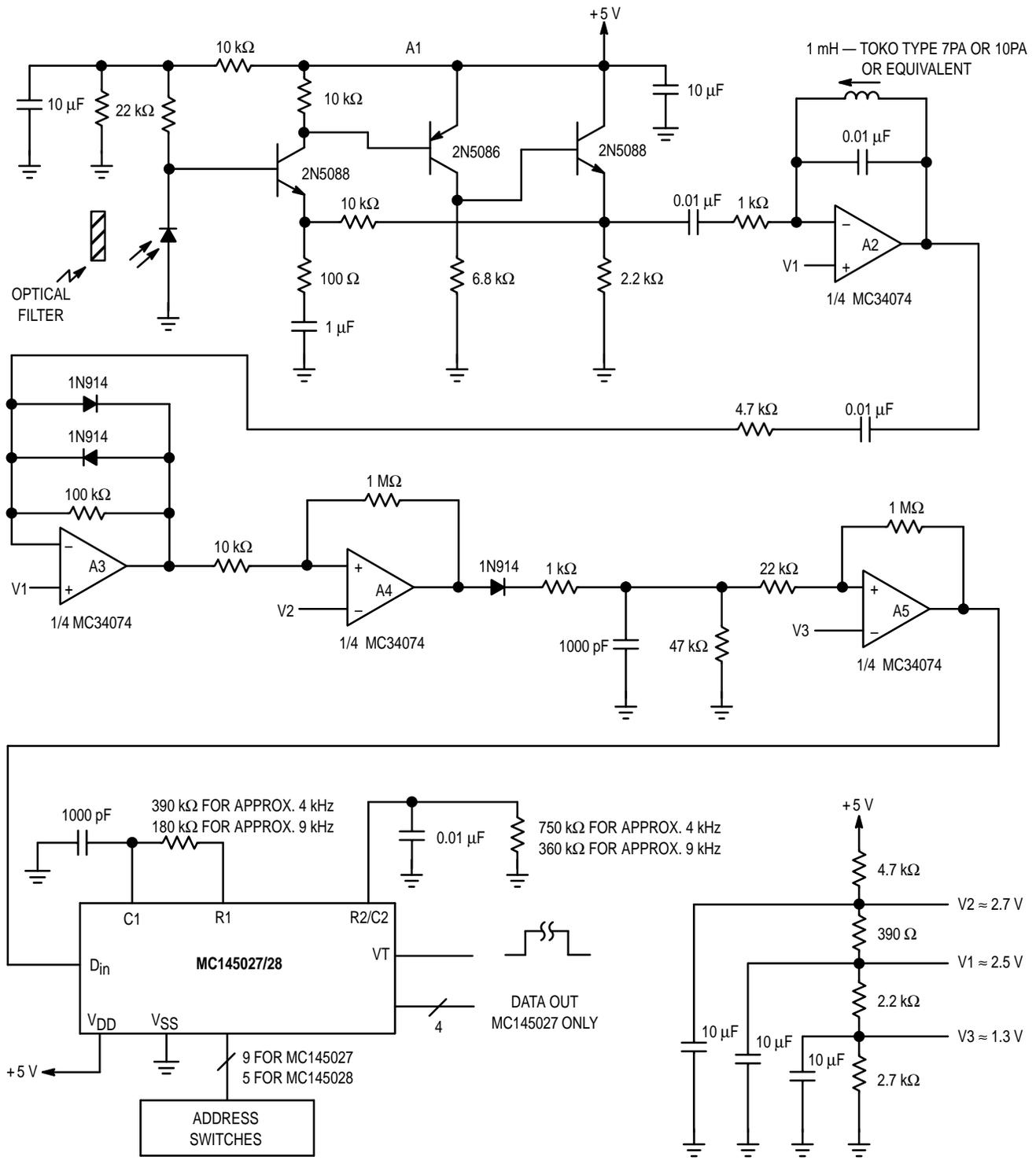
Figure 20. Infrared Receiver
