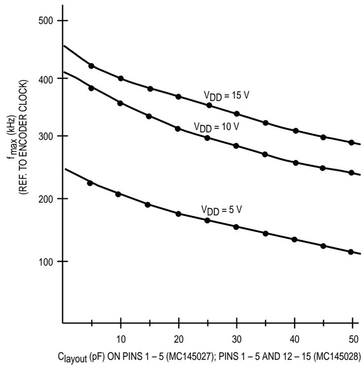
Figure 12.  $f_{max}$  vs  $C_{layout}$  — Decoders Only
