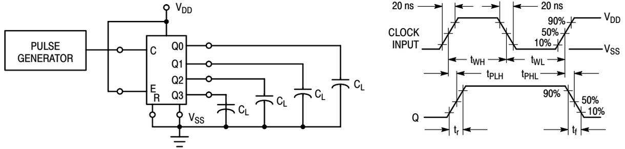
Figure 2. Switching Time Test Circuit and Waveforms
