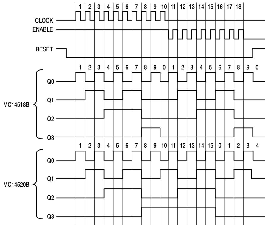
Figure 3. Timing Diagram
