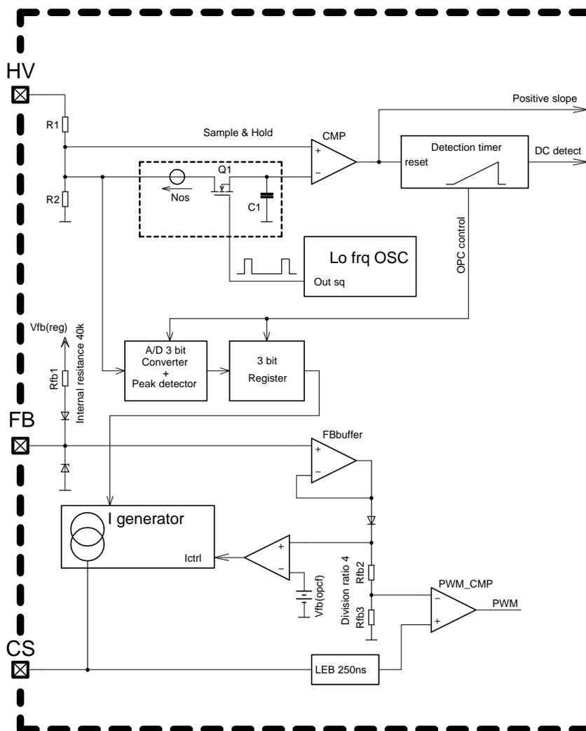
Figure 69. Block Schematic of Overpower Protection Circuit
