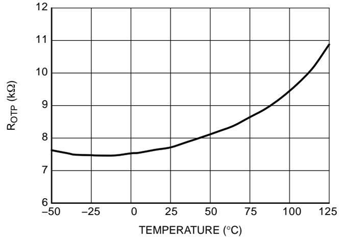
**Figure 20. OTP Resistance Threshold  $R_{OTP}$  at Latch Pin**
