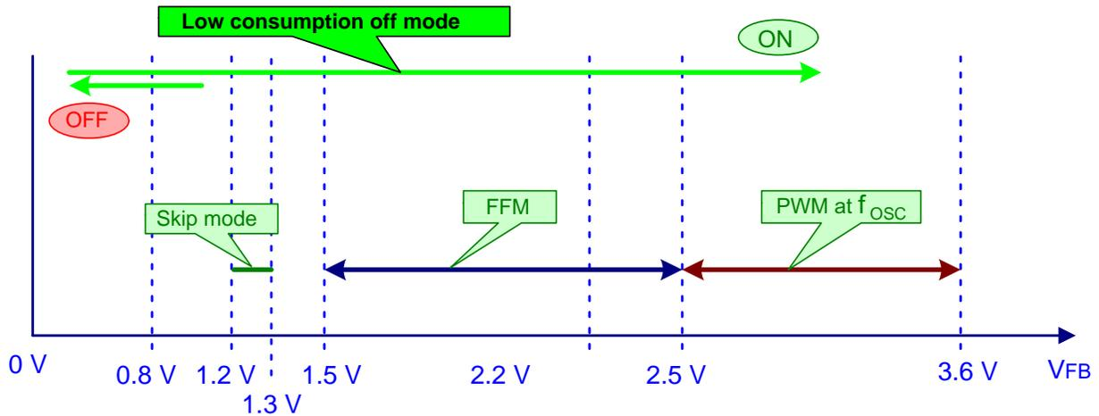
Figure 45. Mode Control with FB Pin Voltage
