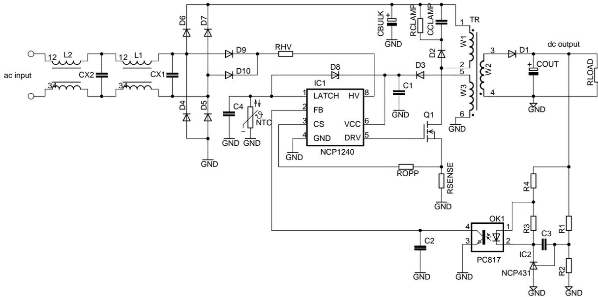
Figure 1. Flyback Converter Application Using the NCP1240
