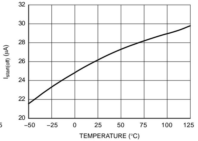
**Figure 4. Off-State Leakage Current I<sub>start(off)</sub>**
