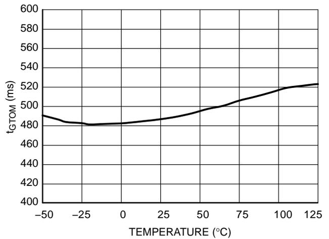
**Figure 44. Go To Off Mode Timer Duration  $t_{GTOM}$**
