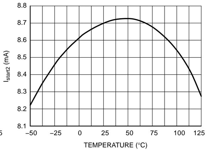
**Figure 6. High Voltage Startup Current Flowing Out of V<sub>CC</sub> Pin I<sub>start2</sub>**
