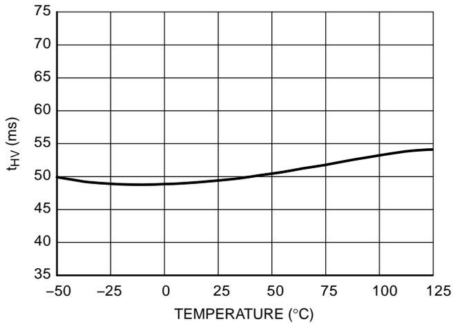
**Figure 41. Timer Duration for Line Cycle Drop-out  $t_{HV}$**
