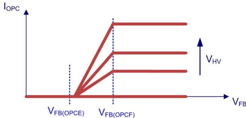
Figure 67. Overpower Protection Current Relation to Feedback Voltage
