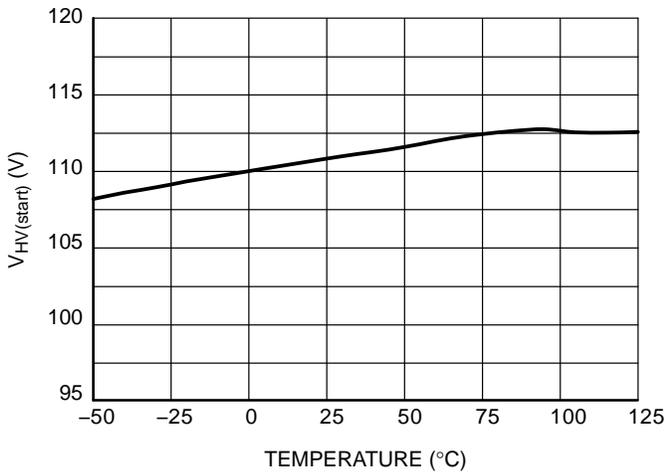
**Figure 7. Brown-out Device Start Threshold**
