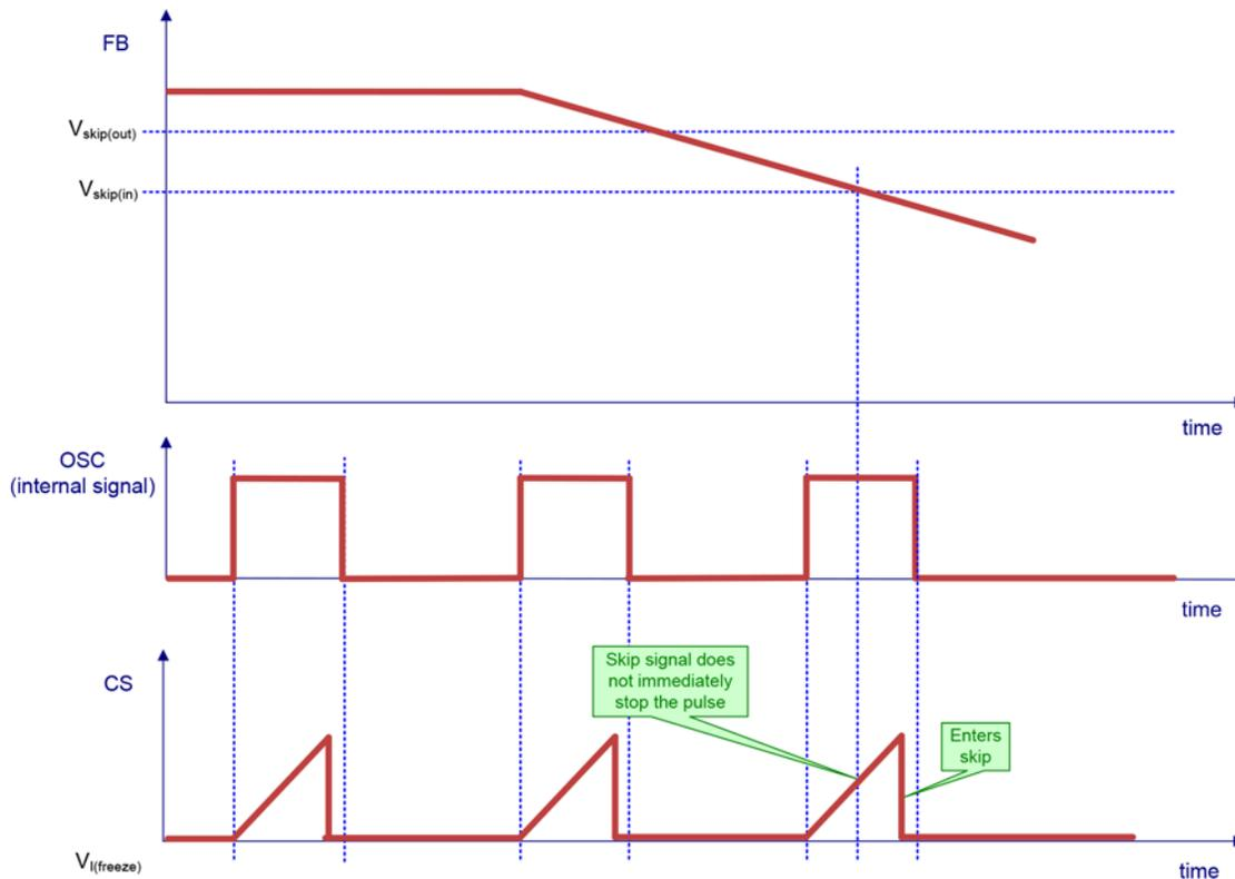
Figure 62. Technique Preventing Short Pulses in Skip Mode
