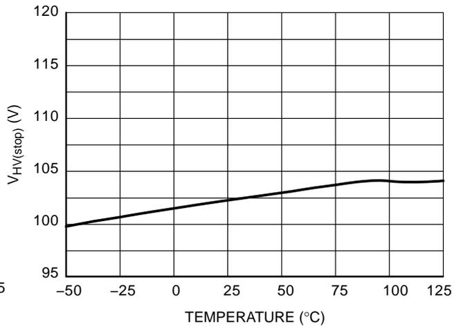
**Figure 8. Brown-out Device Stop Threshold**
