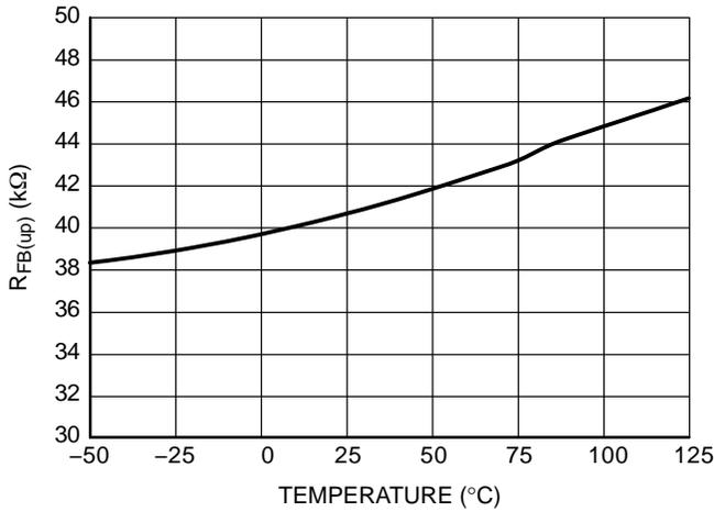
**Figure 15. FB Pin Internal Pull-up Resistor  $R_{FB(up)}$**
