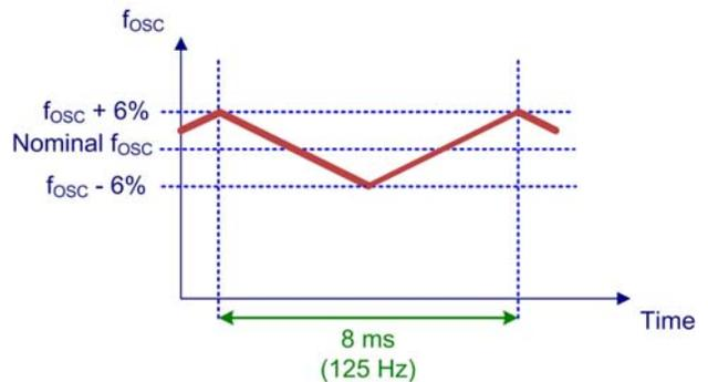
Figure 59. Frequency Modulation of the Maximum Switching Frequency
