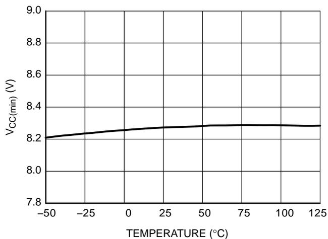
**Figure 34. HV Current Source Restart Threshold  $V_{CC(min)}$**
