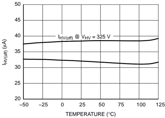
**Figure 5. Off-Mode HV Supply Current I<sub>HV(off)</sub>**
