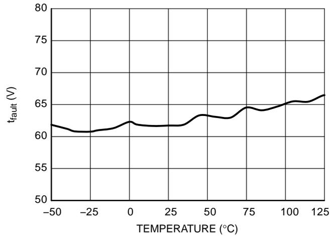
**Figure 42. Fault Timer Duration  $t_{fault}$  (NCP1240A/B only)**
