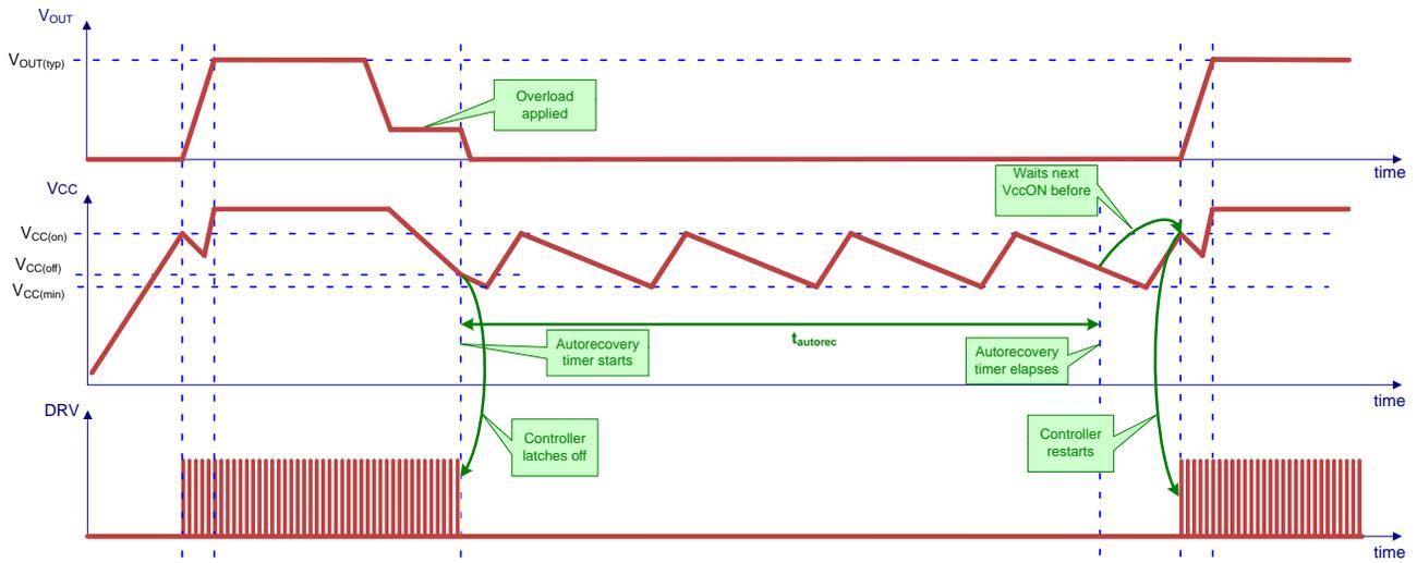
Figure 50.  $V_{CC}$  Collapses After Overload and Its Recovery
