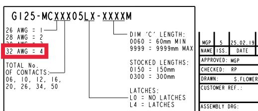
I. LATCHES ARE SHOWN FOR ILLUSTRATION ONLY. WHEN "LO" IS SPECIFIED IN THE ORDER CODE NO LATCHES WILL BE FITTED.
