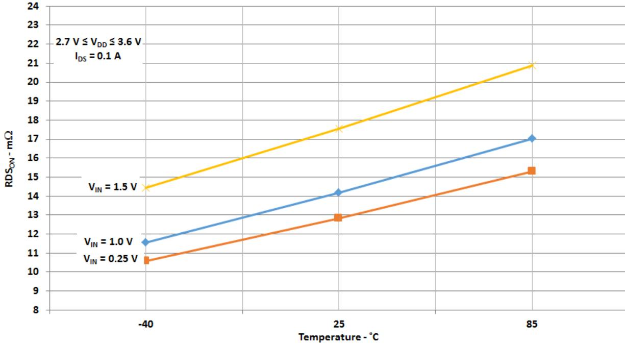
$R_{DS(ON)}$  vs.  $V_{IN}$ , and  $V_{DD}$
