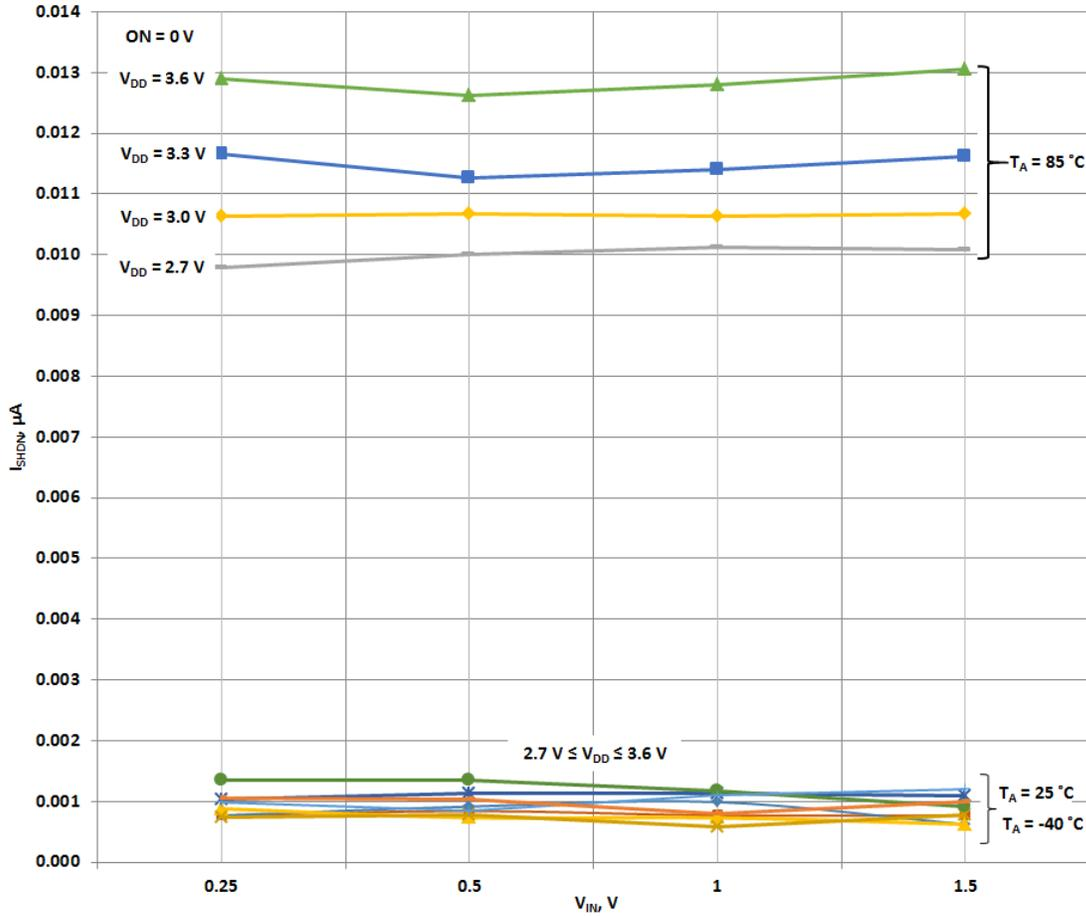
An Ultra-low Power,  $R_{DS(ON)} 18\text{ m}\Omega$ , 1 A,  $0.82\text{ mm}^2$  WLCSP Integrated Power Switch with 550  $\mu\text{s}$  Total Turn-on Time
