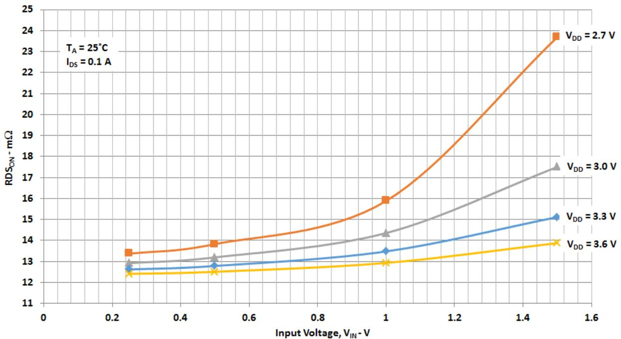
An Ultra-low Power,  $R_{DS(ON)}$  18 m $\Omega$ , 1 A, 0.82 mm<sup>2</sup> WLCSP Integrated Power Switch with 550  $\mu$ s Total Turn-on Time
